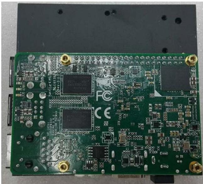
9. Assemble the top cover with UP board with bottom chassis, make sure USB ports align first
