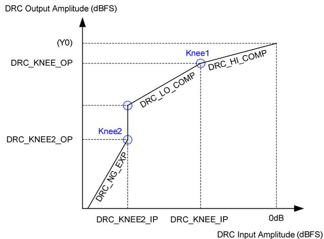
Figure 29 DRC Response Characteristic
