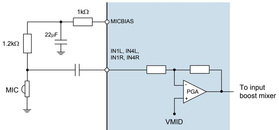
**Figure 97 Microphone Connection, with MICBIAS filter components**
