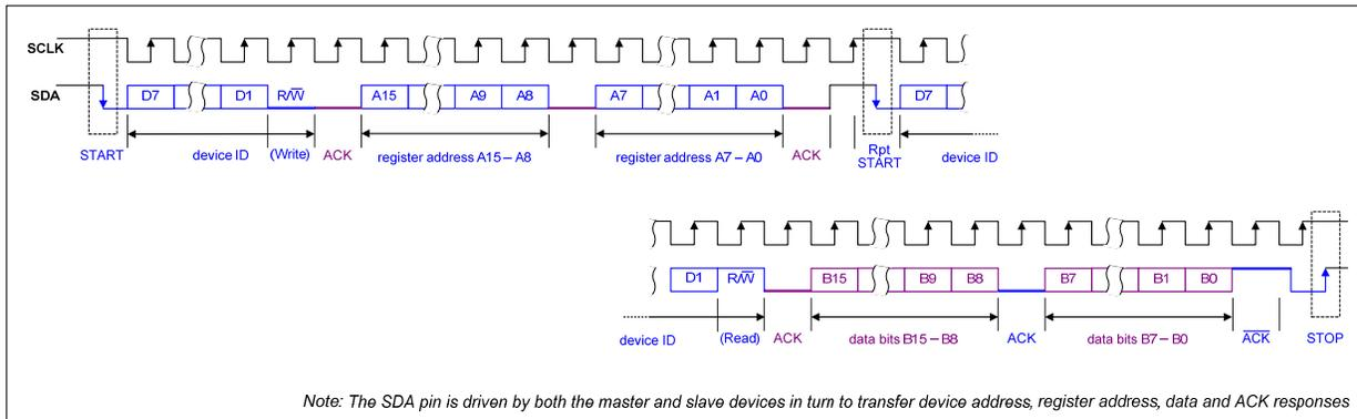
Figure 65 Control Interface 2-wire (I2C) Register Read
