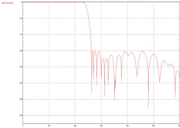
Figure 85 ADC Digital Filter Frequency Response (128OSR)
