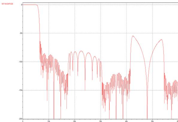
Figure 77 DAC Filter Response for 12k Sample Rate
