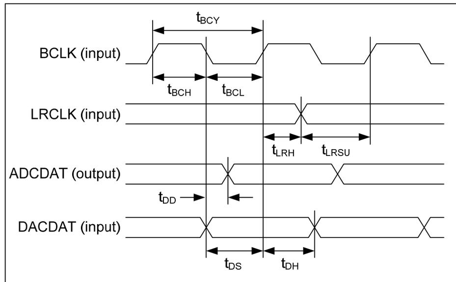
Figure 4 Audio Interface Timing – Slave Mode
