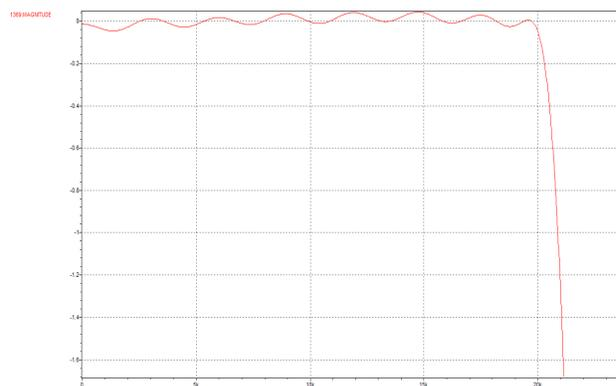
Figure 84 DAC Playback Filter Passband Ripple for 44.1k Sample Rate (MCLK=11.2896MHz)
