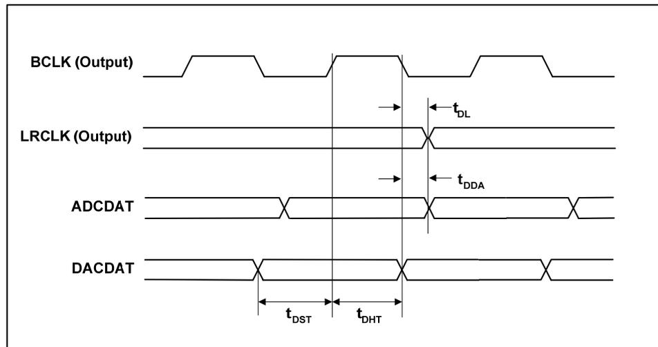
Figure 3 Audio Interface Timing - Master Mode
