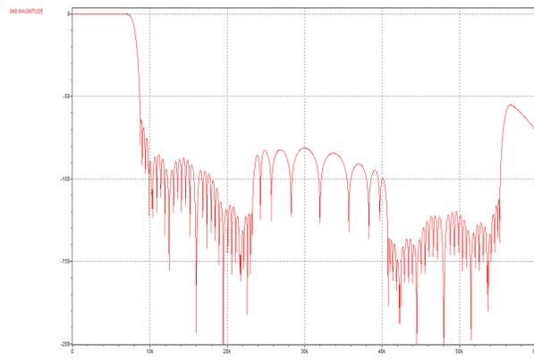
Figure 78 DAC Filter Response for 16k Sample Rate
