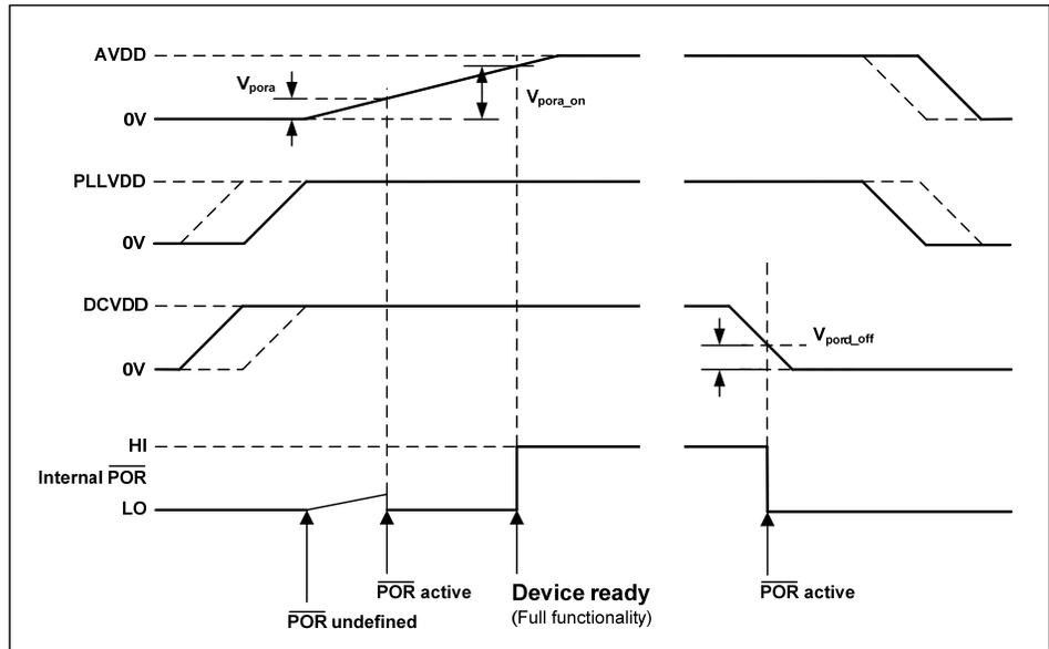
Figure 12 Power On Reset Timing - DCVDD Enabled First
