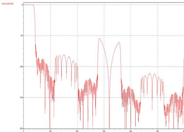
Figure 75 DAC Filter Response 8k Sampling Rate
