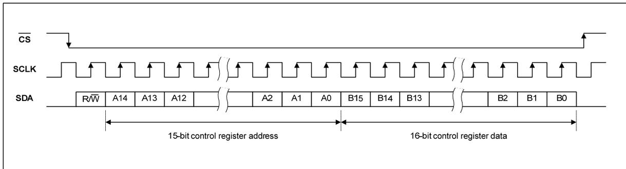
Figure 71 3-Wire Serial Control Interface
