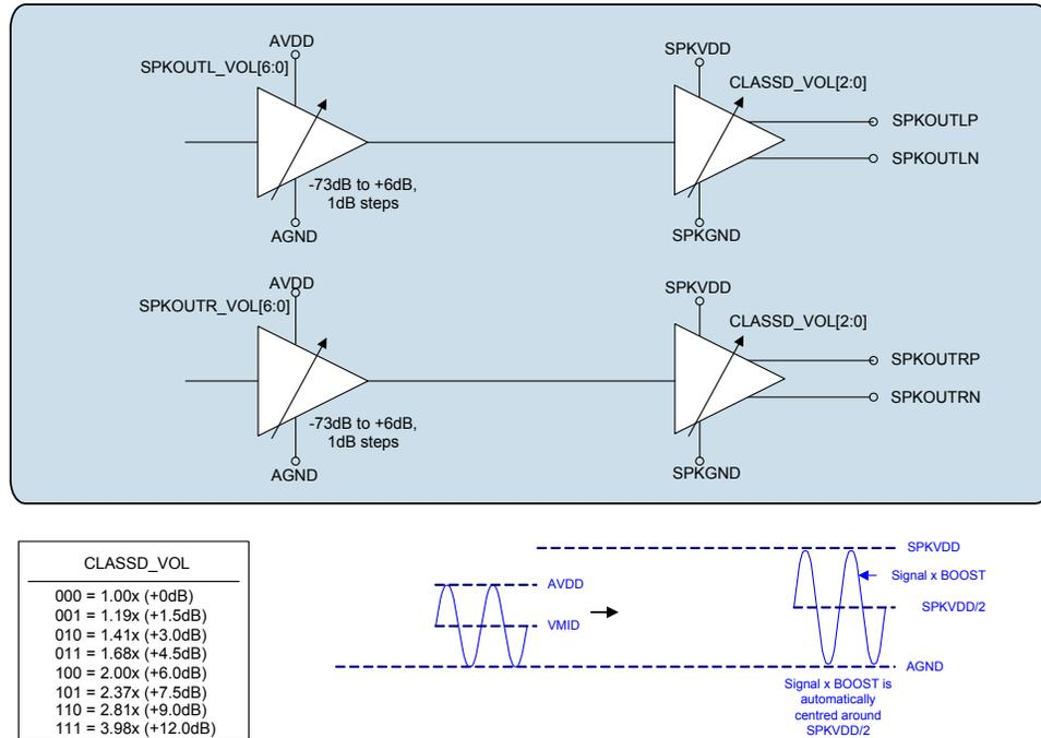
Figure 36 Speaker Output Configuration and AC Boost Operation
