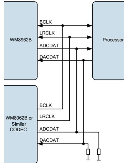
**Figure 42 TDM with Other CODEC as Master**
