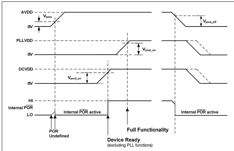
Figure 11 Power On Reset Timing - AVDD Enabled First
