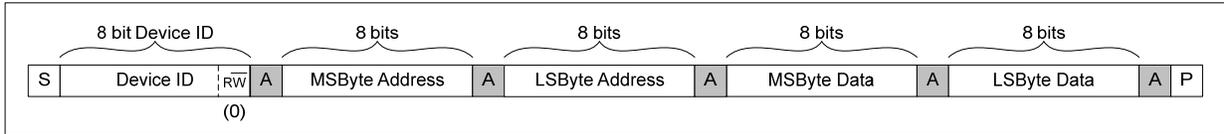
Figure 66 Single Register Write to Specified Address
