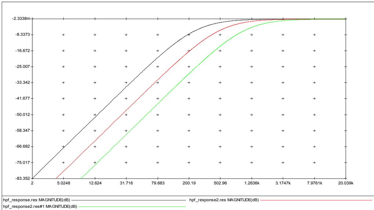
Figure 88 ADC Digital High Pass Filter Ripple (48kHz, Voice Mode, ADC\_HPF\_CUT=01, 10 and 11)
