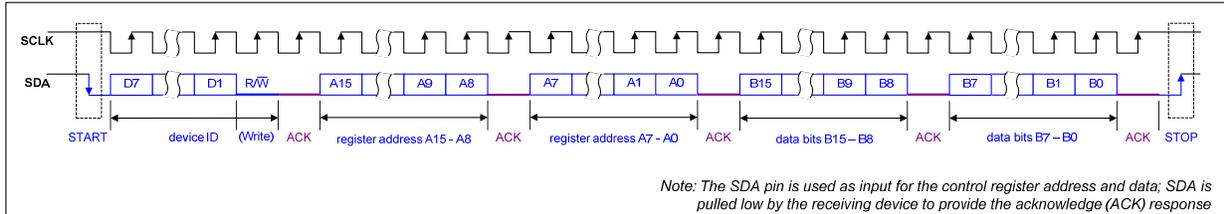
Figure 64 Control Interface 2-wire (I2C) Register Write
