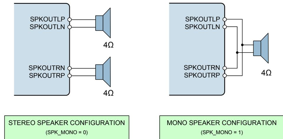
**Figure 35 Mono and Stereo Speaker Output Configuration**
