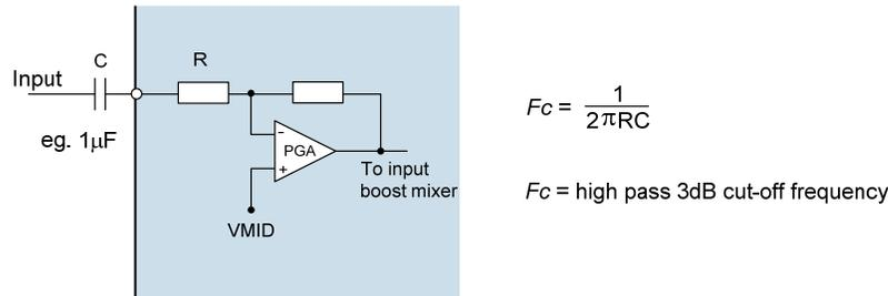
**Figure 95 Audio Input Path DC Blocking Capacitor**
