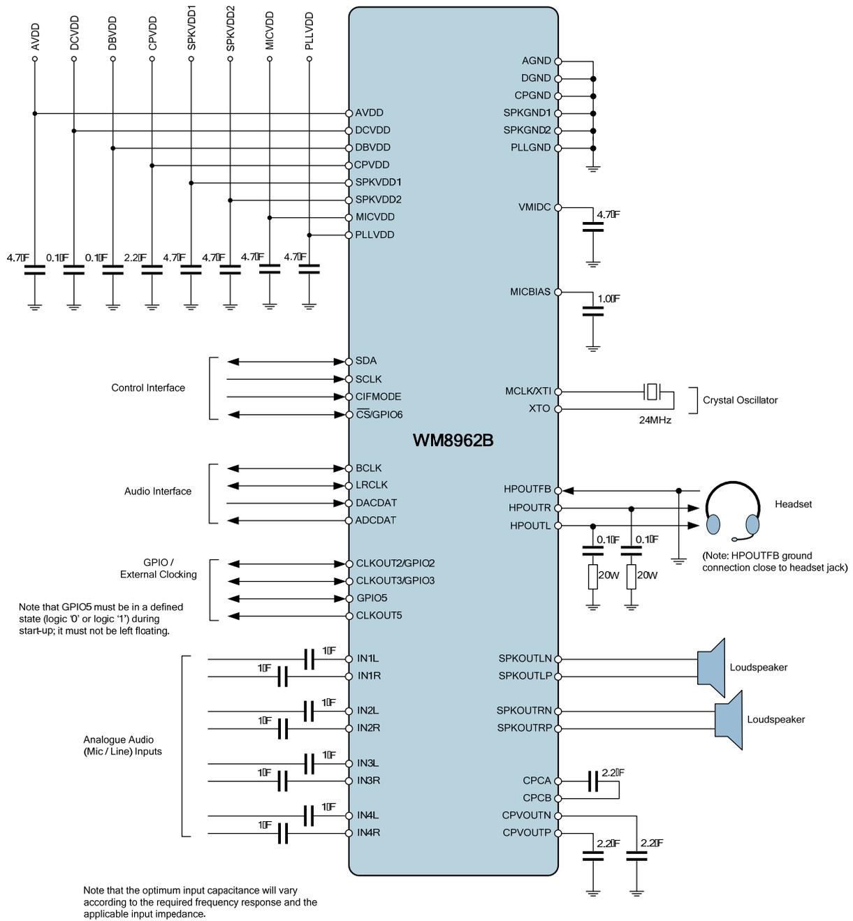
Figure 98 WM8962B Recommended External Components
