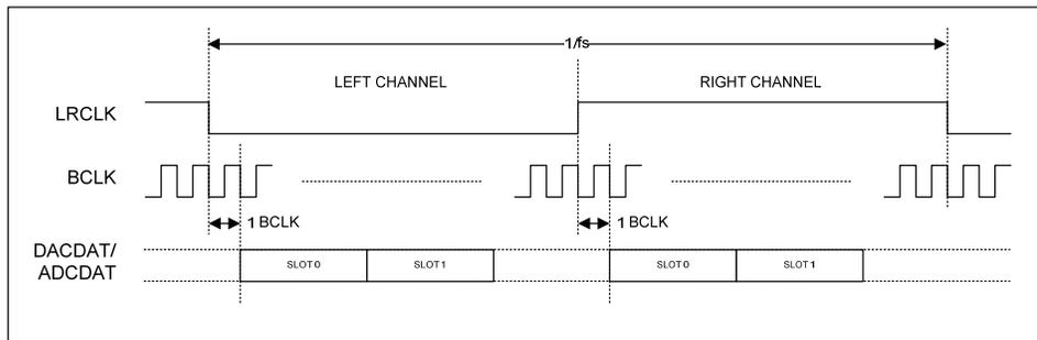
Figure 53 TDM in I<sup>2</sup>S Mode
