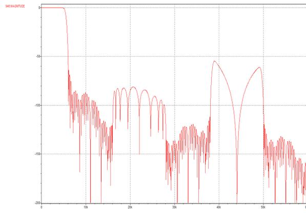
Figure 76 DAC Filter Response for 11.025k Sample Rate
