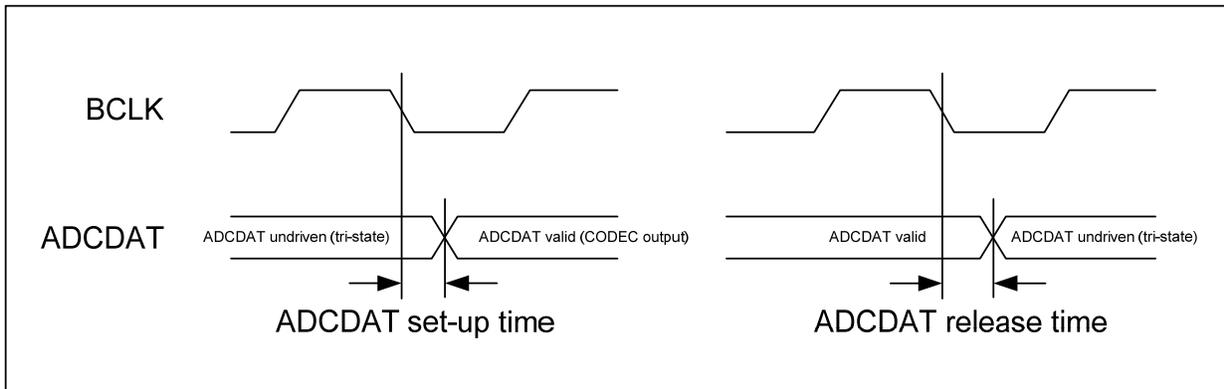
Figure 5 Audio Interface Timing – TDM Mode
