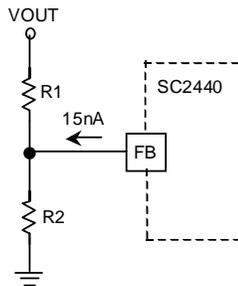
Figure 4.  $V_{OUT}$  is set with a Resistive Divider
