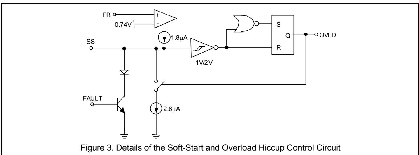
Figure 3. Details of the Soft-Start and Overload Hiccup Control Circuit
