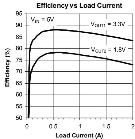
Figure 17(a). 1.3MHz 5V to 3.3V and 1.8V Step-down Converter
