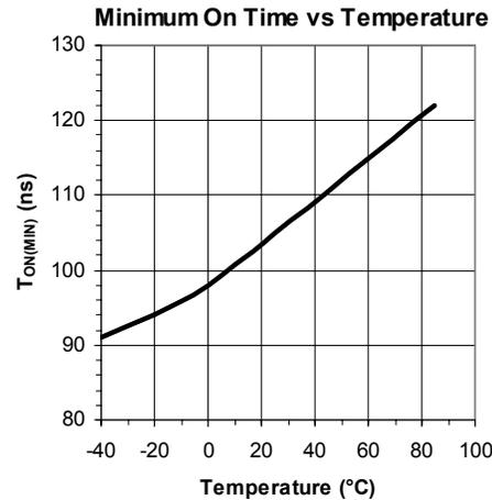
Figure 6. Variation of Minimum On Time with Temperature.
