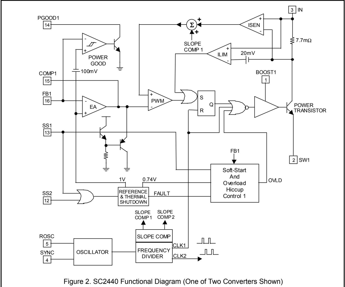
Figure 2. SC2440 Functional Diagram (One of Two Converters Shown)
