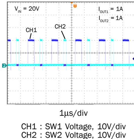
Figure 19(b). Switching Waveforms.
