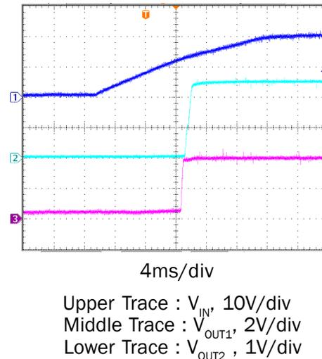
Figure 19(c).  $V_{IN}$  Start Up Transient.  $I_{OUT1} = I_{OUT2} = 1.5A$ .
