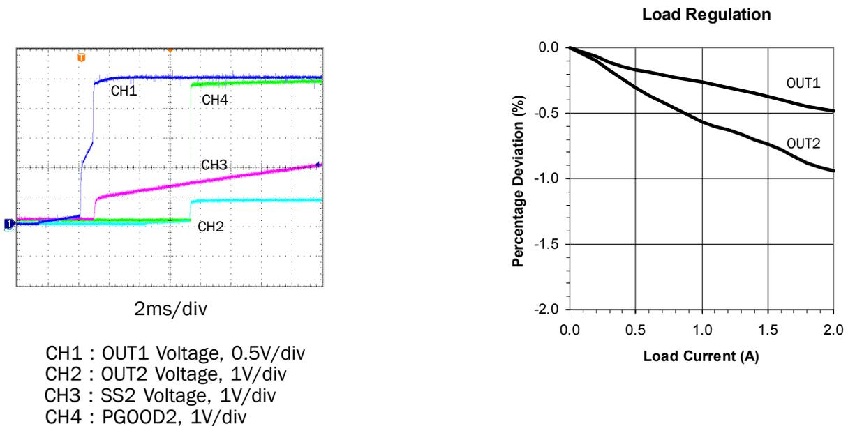
Figure 18(b).  $V_{IN}$  Start-up Transient ( $I_{OUT1} = I_{OUT2} = 1A$ ).
