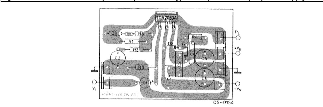
Figure 19. Bridge amplifier with split power supply ( $P_O = 34\text{ W}$ ,  $V_S = \pm 16\text{ V}$ )
