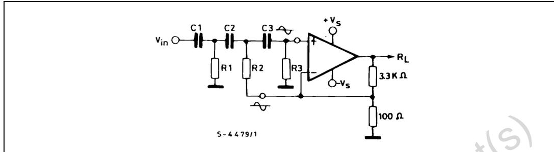
The proposed circuit can realize combined power amplifiers and 12 dB/octave or 18 dB/octave high-pass or low-pass filters.
