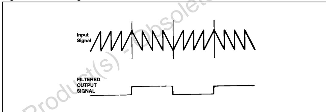
In the case of the sawtooth in [Figure 27](#) the mean level was increased by the TIM distortion, for a sawtooth in the other direction, the opposite is true. The result is an AC signal at the output whose peak-to-peak value is the TIM voltage, which can be measured easily with an oscilloscope. If the peak-to-peak value of the signal and the peak-to-peak of the inverting sawtooth are measured, the TIM can be found very simply from:
