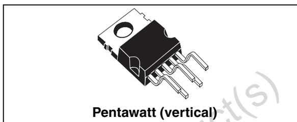
The TDA2030A provides high output current and has very low harmonic and crossover distortion. The device incorporates a short-circuit protection system comprising an arrangement for automatically limiting the dissipated power so as to keep the operating point of the output transistors within their safe operating range. A conventional thermal shutdown system is also included.
