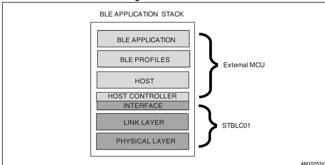
**Figure 2. Simplified application diagram**
