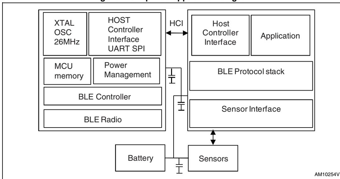
The protocol stack running in the host is released separately in the form of static library for the STM32L. BLE qualified profiles are available separately.
