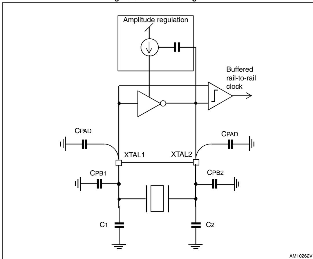
Low power consumption and fast startup time is achieved by choosing a quartz crystal with a low load capacitance  $C_0$ . A reasonable choice for capacitor  $C_0$  is 10 pF. The Xtal startup time is typically 1 ms but can go up to 10 ms depending on the quality factor of the external quartz chosen. To achieve good frequency stability, the following equation then needs to be satisfied:
