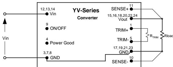
Figure 17. Programming Output Voltage With A Resistor
