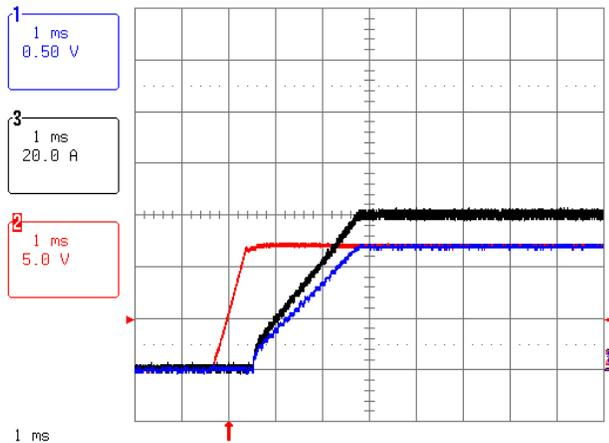
**Figure 11. Typical Start-Up with application of Vin**
