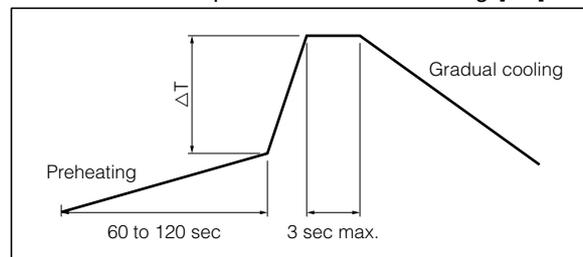
ΔT : Allowable temperature difference  $\Delta T \leq 150 \text{ }^\circ\text{C}$
