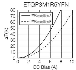
PWB condition A : FR4, single layer PWB, t=1.6mm \*our specification
