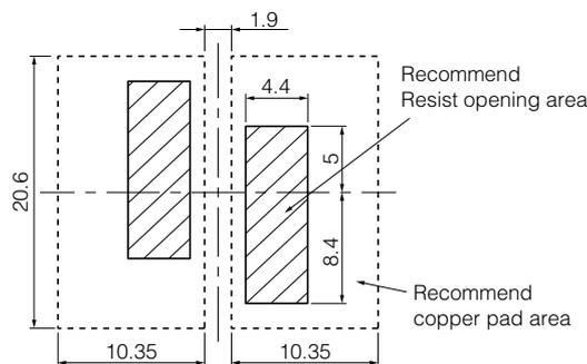
\* Due to bigger part, Thermal Capacity is large and may occur PWB temperature differences during reflow process. Recommended land pattern (Heat absorb) should be designed with reflow mountability.
