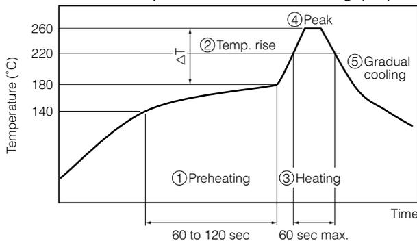
The rapid cooling (forced cooling) during Gradual cooling part should be avoided, because this may cause defects such as the thermal cracks, etc.
