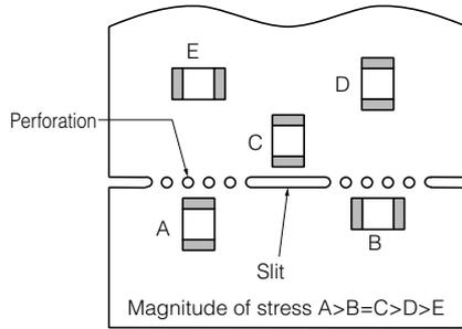
(3) The magnitude of mechanical stress applied to the Inductors when the circuit board is divided is in the order of push back < slit < V-groove < perforation.
