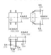
Terminal thickness = 0.15.006General tolerance:  $\pm 0.1 \pm .004$
