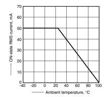
1-(3). ON-state RMS current vs. ambient temperature characteristics
