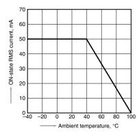
1-(2). ON-state RMS current vs. ambient temperature characteristics
