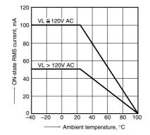
2. On voltage vs. ambient temperature characteristics
