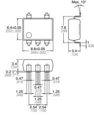
Terminal thickness = 0.25.010General tolerance:  $\pm 0.1 \pm .004$
