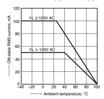
1-(6). ON-state RMS current vs. ambient temperature characteristics
