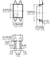
Terminal thickness = 0.20.008General tolerance:  $\pm 0.1 \pm .004$
