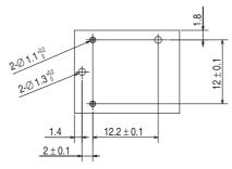
Terminal Arrangement/Internal Connections (Bottom View)
