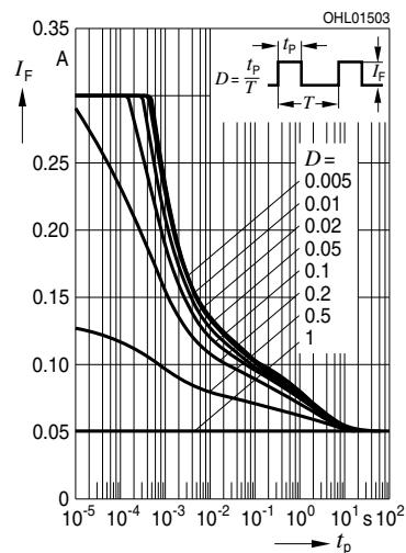
**Permissible Pulse Handling Capability****Zulässige Impulsbelastbarkeit  $I_F = f(t_p)$** D: Duty cycle,  $T_S = 85^\circ\text{C}$
