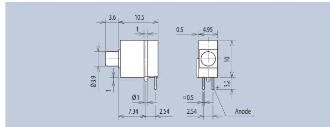
These components with lateral fins and grooves, which interlock when being stacked, guarantee appropriate stabilization on the printed circuit board. With an integrated protective resistor this component is suitable for low-current applications, too. Divers operating voltages are available.
