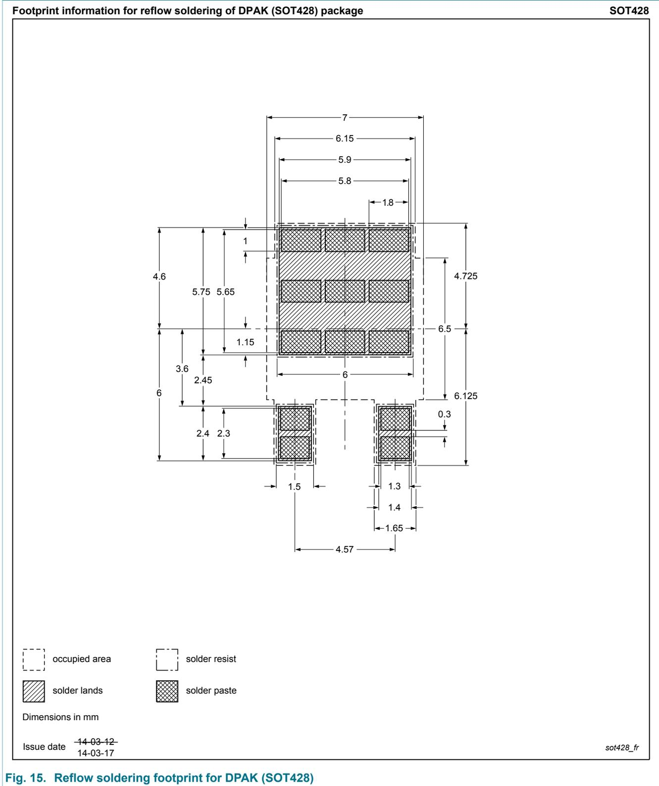
Fig. 15. Reflow soldering footprint for DPAK (SOT428)
