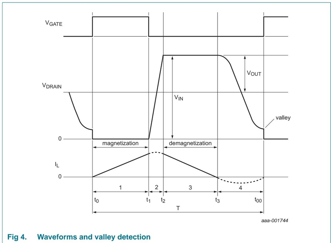
Fig 4. Waveforms and valley detection
