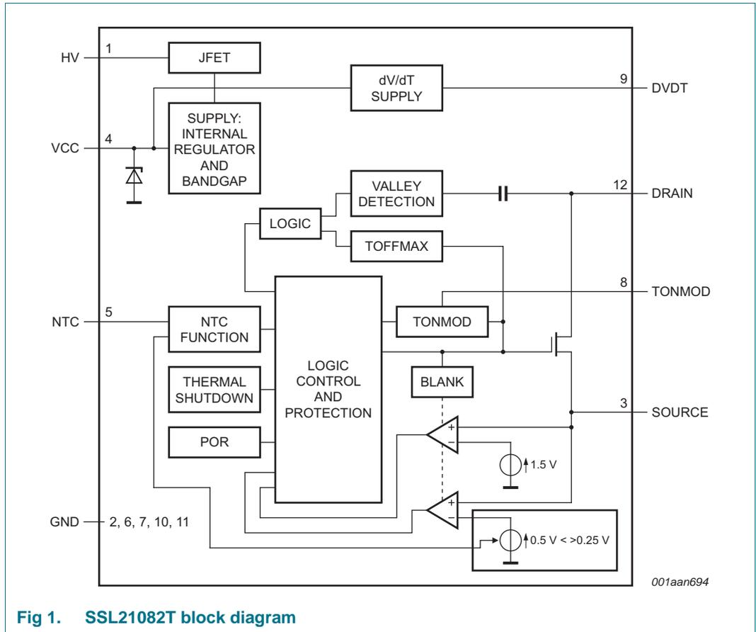
Fig 1. SSL21082T block diagram
