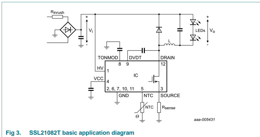
Fig 3. SSL21082T basic application diagram
