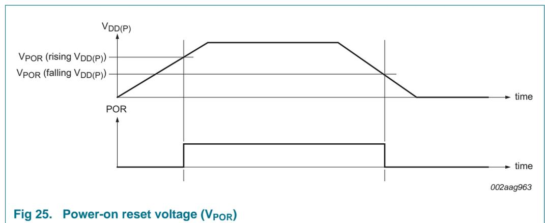
**Fig 25. Power-on reset voltage (V<sub>POR</sub>)**
