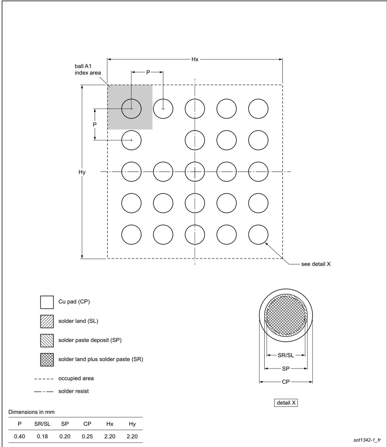
Fig 47. PCB footprint for SOT1342-1 (XFBGA24); reflow soldering
