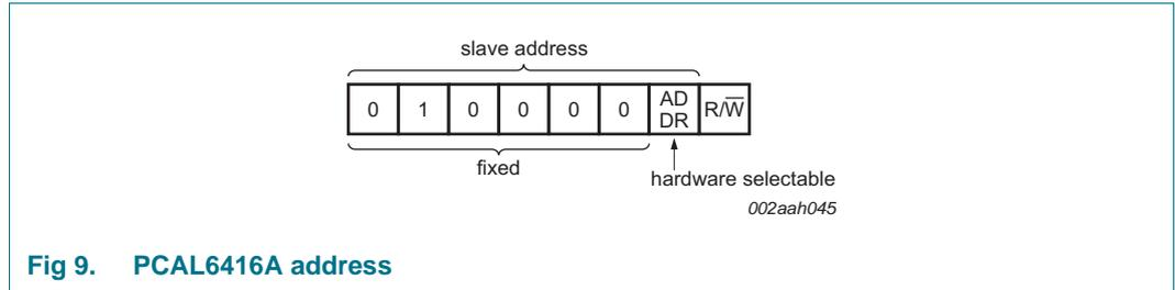
ADDR is the hardware address package pin and is held to either HIGH (logic 1) or LOW (logic 0) to assign one of the two possible slave addresses. The last bit of the slave address (R/W) defines the operation (read or write) to be performed. A HIGH (logic 1) selects a read operation, while a LOW (logic 0) selects a write operation.
