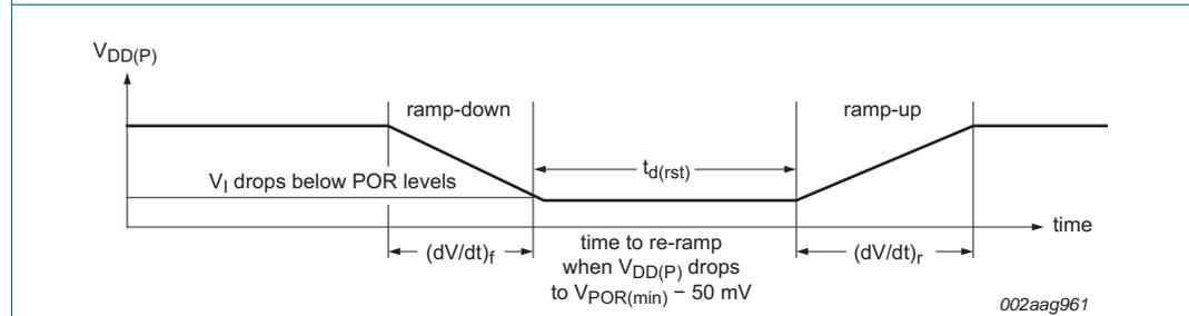
Fig 23.  $V_{DD(P)}$  is lowered below the POR threshold, then ramped back up to  $V_{DD(P)}$
