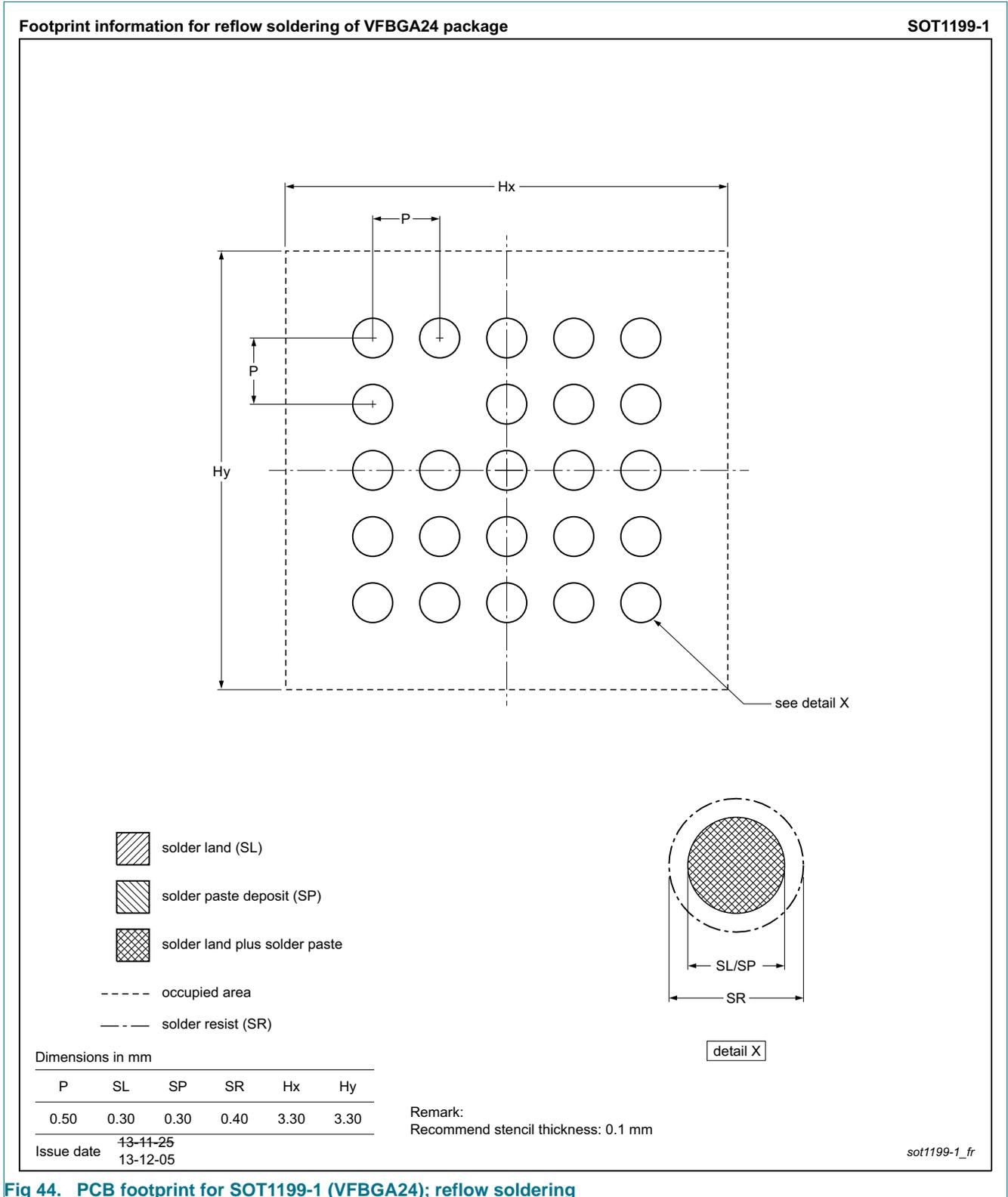
Fig 44. PCB footprint for SOT1199-1 (VFBGA24); reflow soldering
