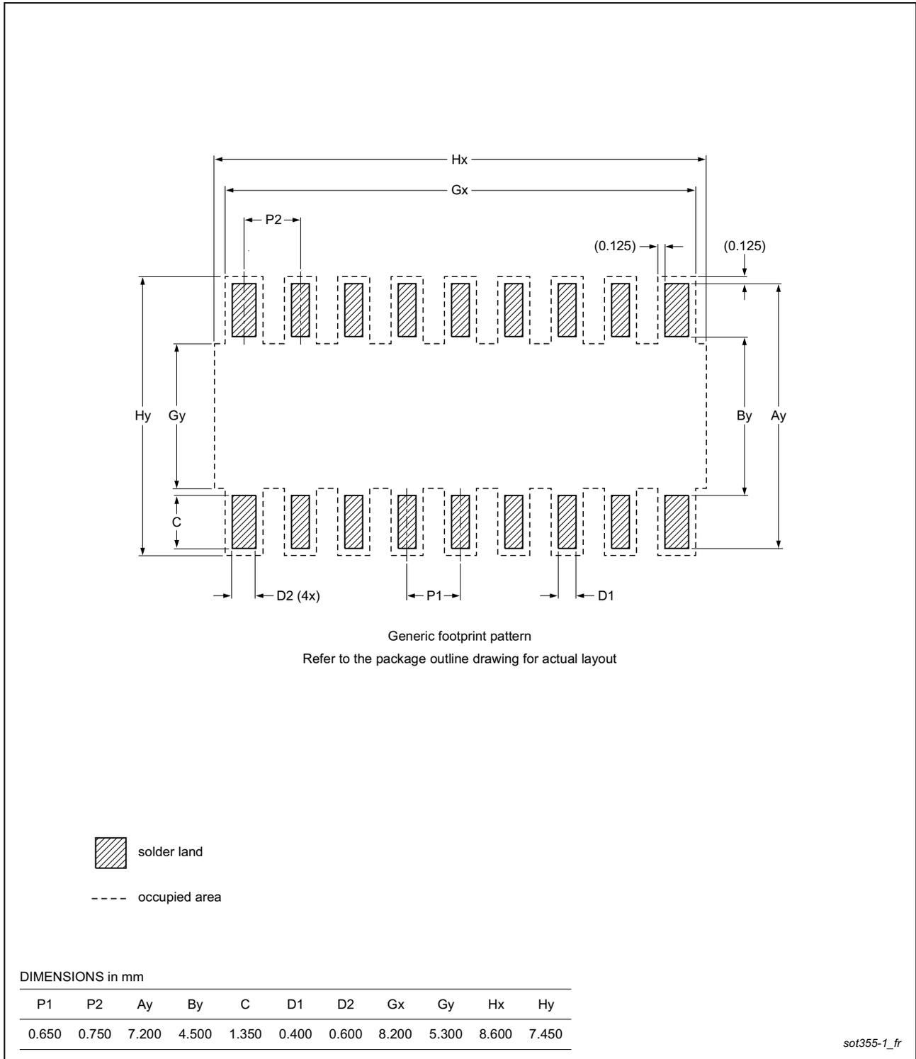
Fig 45. PCB footprint for SOT355-1 (TSSOP24); reflow soldering
