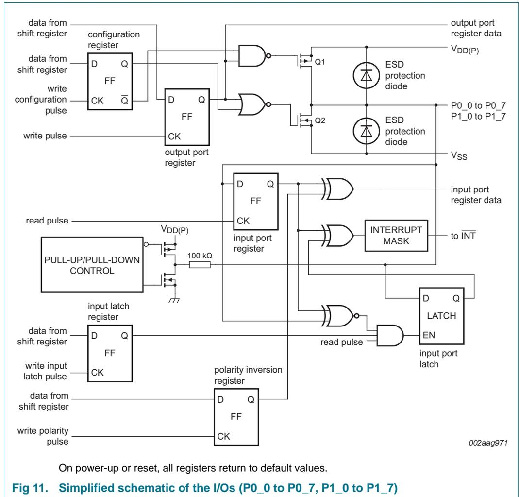
Fig 11. Simplified schematic of the I/Os (P0\_0 to P0\_7, P1\_0 to P1\_7)
