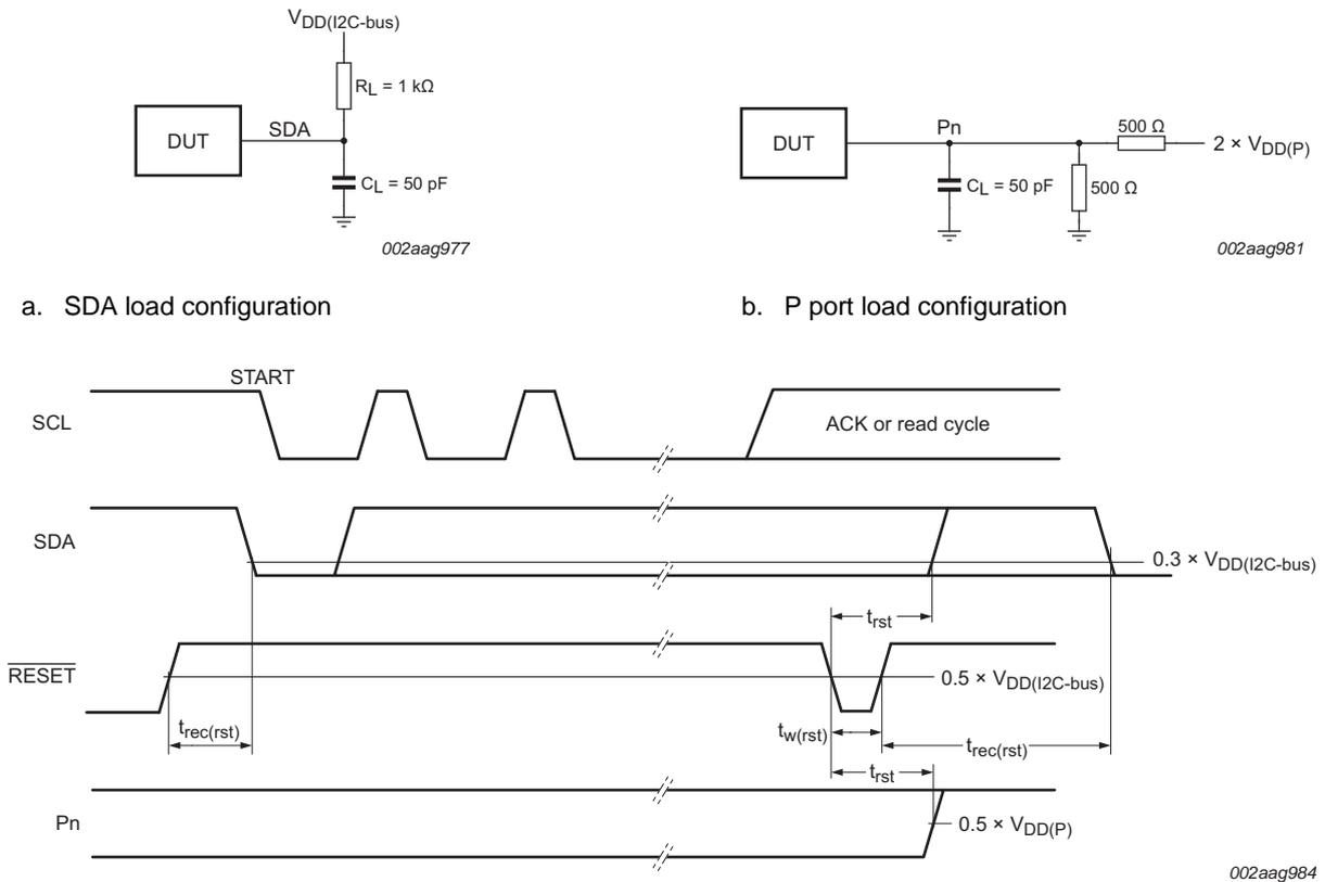
**Fig 37. Reset load circuits and voltage waveforms**
