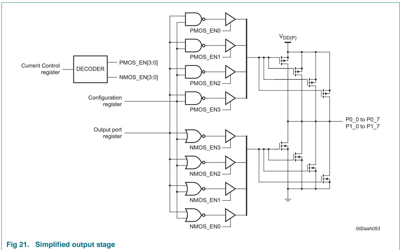
**Fig 21. Simplified output stage**
