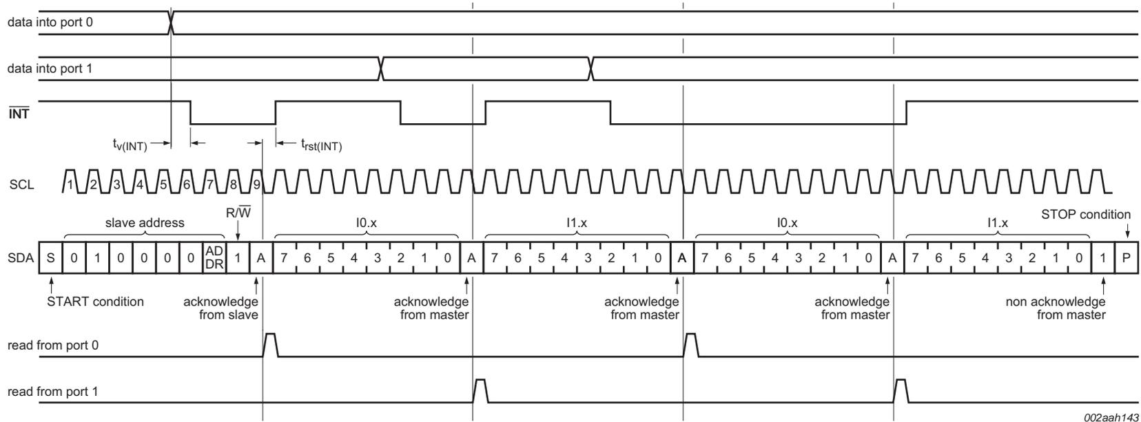
**Remark:** Transfer of data can be stopped at any moment by a STOP condition. When this occurs, data present at the latest acknowledge phase is valid (output mode). It is assumed that the command byte has previously been set to '00' (read input port register).
