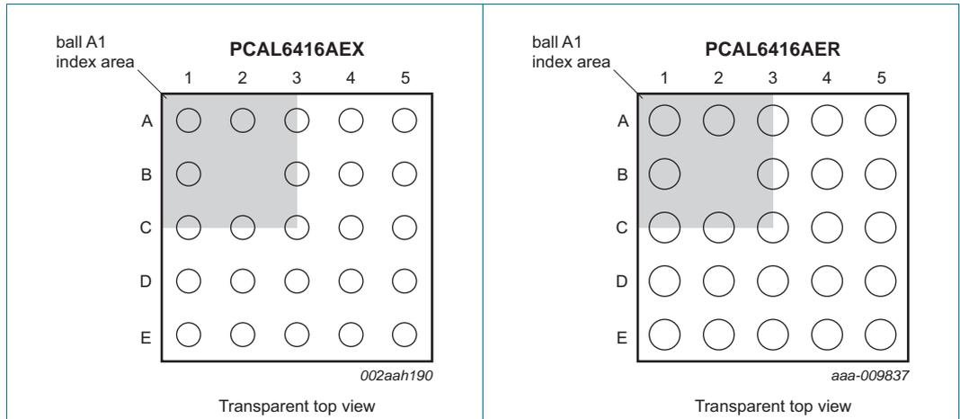
**Fig 6. Pin configuration for XFBGA24 (2 mm × 2 mm); EX option**
