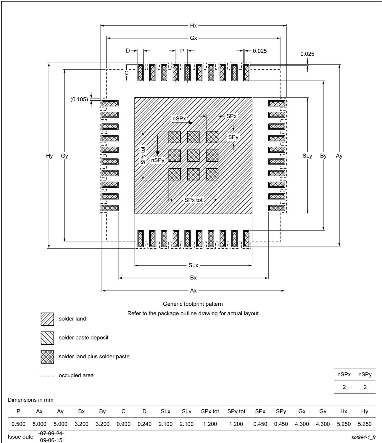
Fig 46. PCB footprint for SOT994-1 (HVQFN24); reflow soldering
