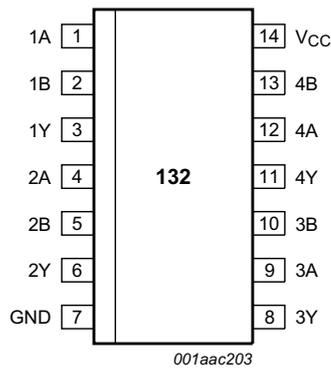
Fig 4. Pin configuration SO14 and (T)SSOP14
