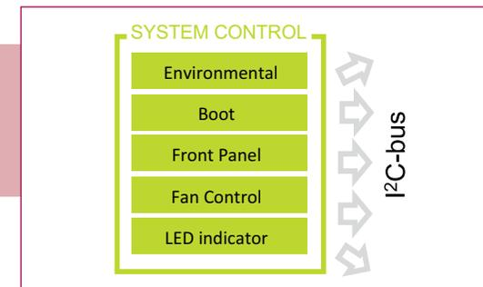
For notebook system control, our I<sup>2</sup>C and SMBus portfolio includes an industry-leading selection of peripherals that enable a variety of functions. There are general-purpose I/O (GPIO) for bus expansion, bus buffers for support of extra devices, level translators for bus-voltage translation, temperature sensors for thermal management, LED drivers for LED control, and ADC/DACs for analog and audio control.
