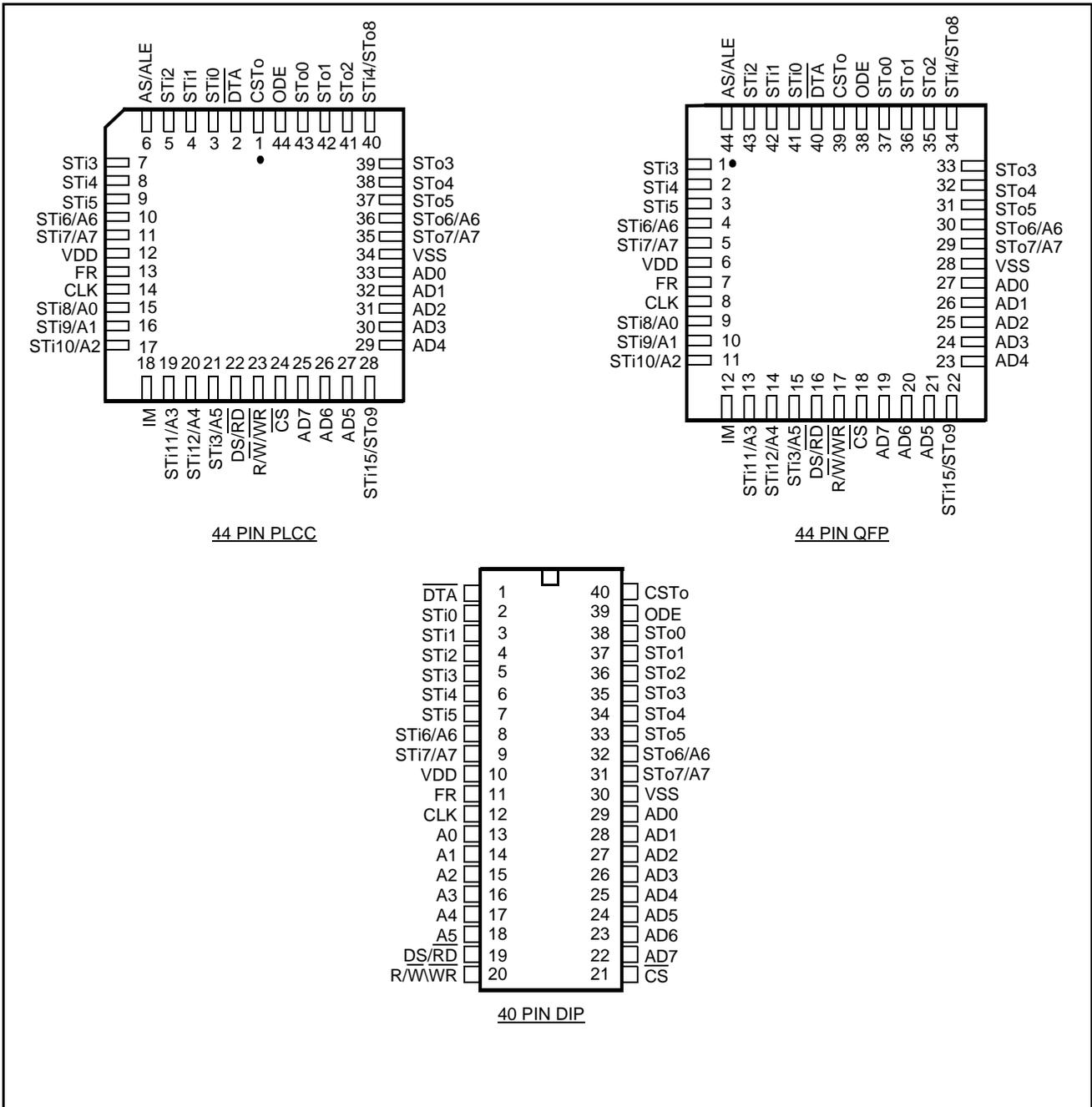
**Figure 2 - Pin Connections**
