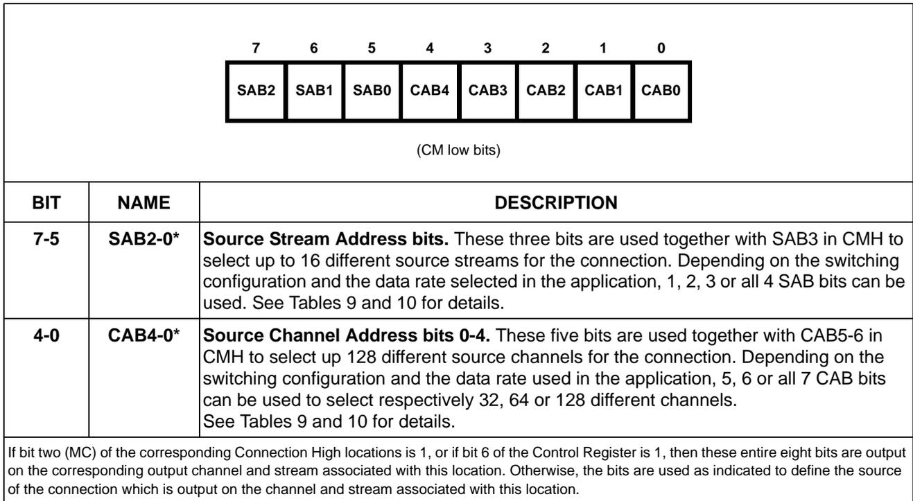
Figure 6 - Connection Memory Low (CML) Bits
