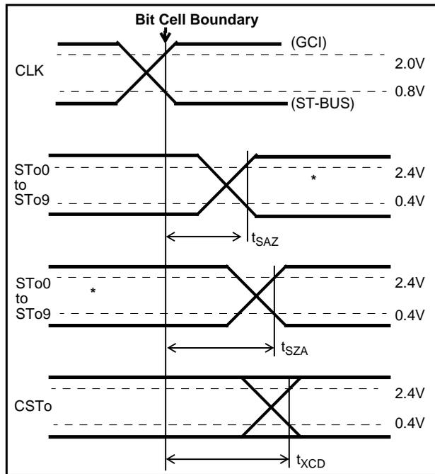
**Figure 18 - Serial Outputs and External Control**
