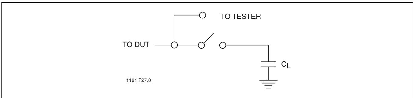
FIGURE 24: A Test Load Example (PP Mode)
