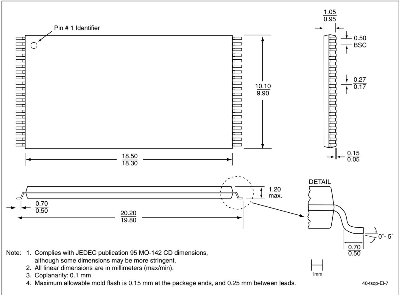
**FIGURE 31: 40-lead Thin Small Outline Package (TSOP) 10mm x 20mm
