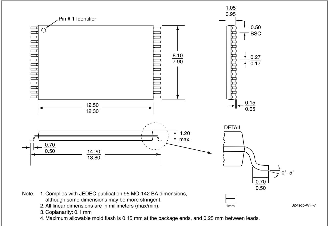
**FIGURE 30: 32-lead Thin Small Outline Package (TSOP) 8mm x 14mm**
