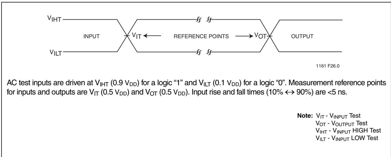
FIGURE 23: AC Input/Output Reference Waveforms (PP Mode)
