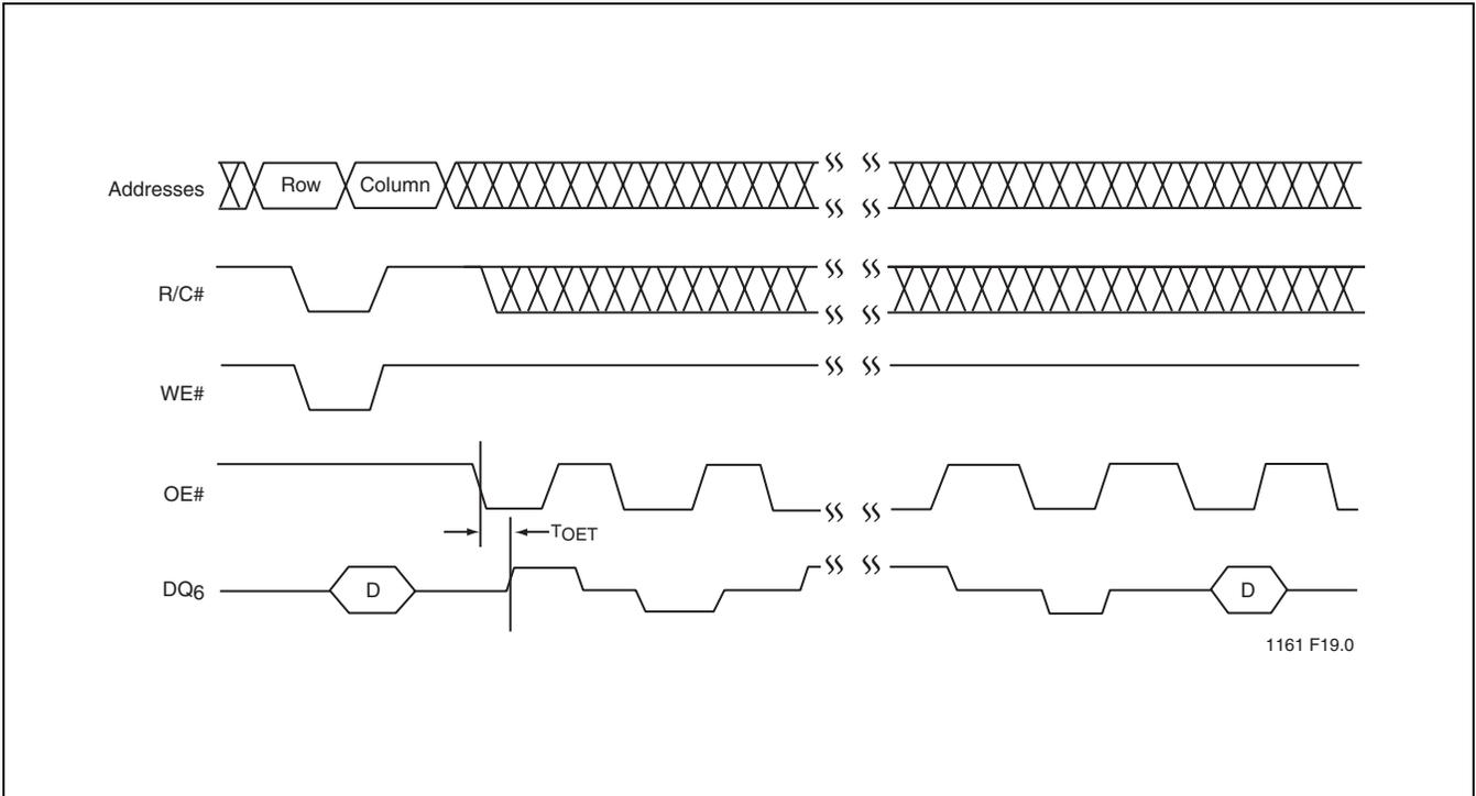
FIGURE 16: Toggle Bit Timing Diagram (PP Mode)
