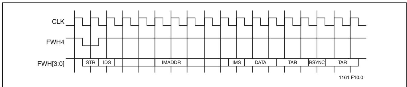
FIGURE 7: Write Waveforms
