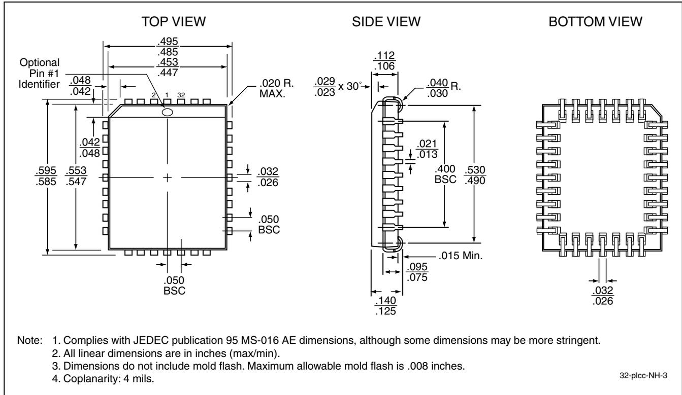
**FIGURE 29: 32-lead Plastic Lead Chip Carrier (PLCC)**
