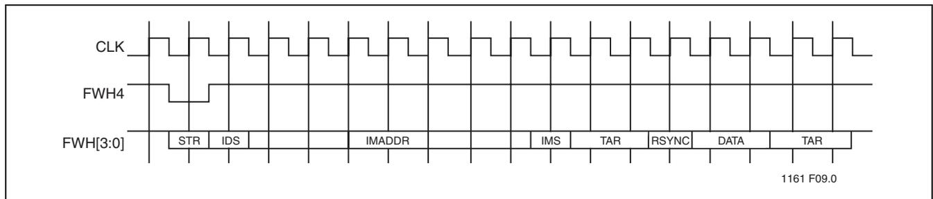
**FIGURE 6: Single-Byte Read Waveforms**
