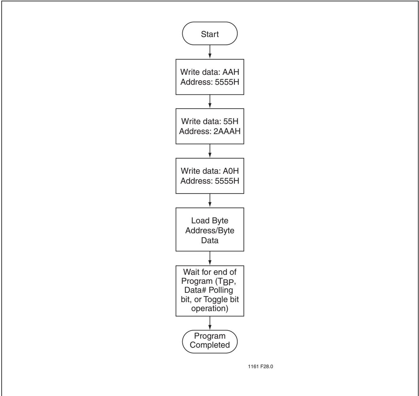
FIGURE 25: Byte-Program Algorithm
