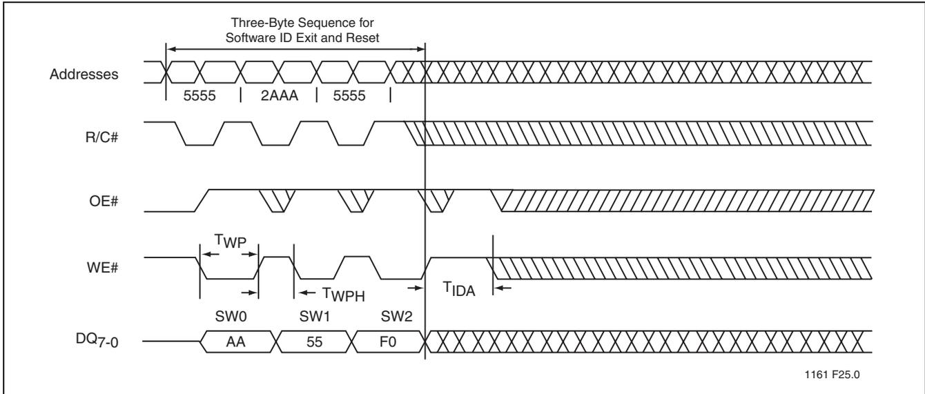
FIGURE 22: Software ID Exit and Reset (PP Mode)
