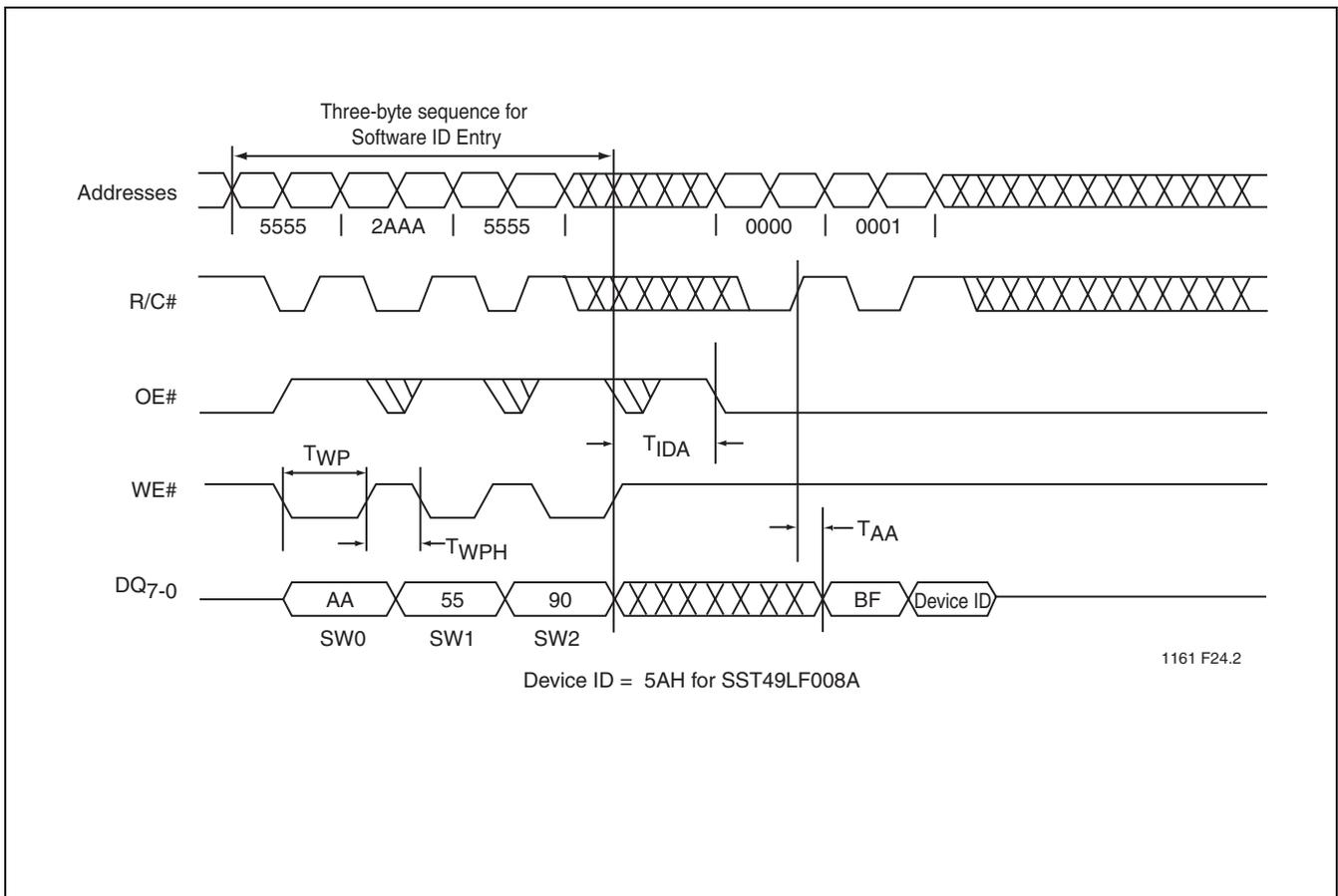
FIGURE 21: Software ID Entry and Read (PP Mode)
