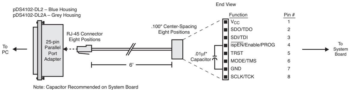
**Figure 6. Programming Cable In-System Programming Interface for the PC (HW7265-DL2 or HW7265-DL2A)**
