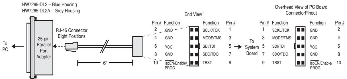
1. For reference purposes, the 2x10 connector on the HW7265-DL2 or HW7265-DL2A is equivalent to Tyco 102387-1. This will interface to standard 100-mil spacing 2x5 headers, or a 2x5 keyed, recessed male connector such as the 3M N2510-5002RB.
