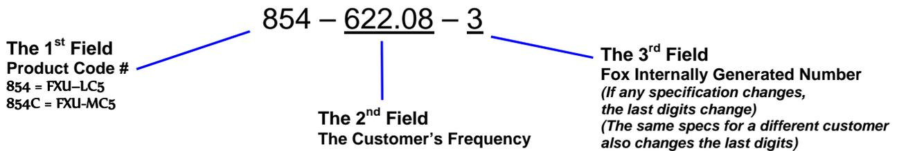
This example, **FXU-LC535R-622.08** = LVDS Output, Ceramic, 5 x 3.2mm Package, 3.3V, ±50 PPM Stability, -40 to +85°C Temperature Range, at 622.08 MHz
