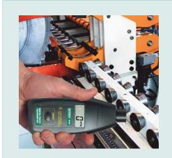
Non-contact measurement on machinery where access is limited
