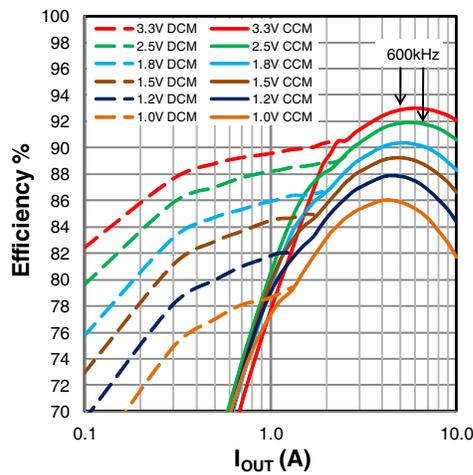
Figure 21: Efficiency,  $V_{IN}=12V$
