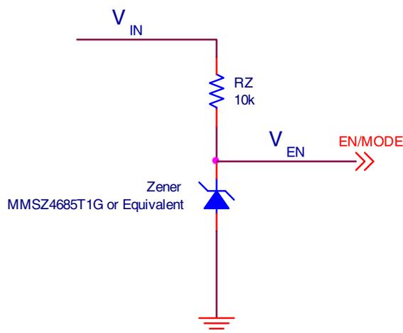
Figure 26: Selecting DCM/CCM by deriving EN/MODE from  $V_{IN}$
