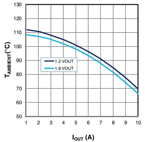
Figure 24: Maximum  $T_{AMBIENT}$  vs  $I_{OUT}$ ,  $V_{IN}=19.6V$
