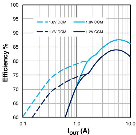
Figure 23: Efficiency,  $V_{IN}=19.6V$
