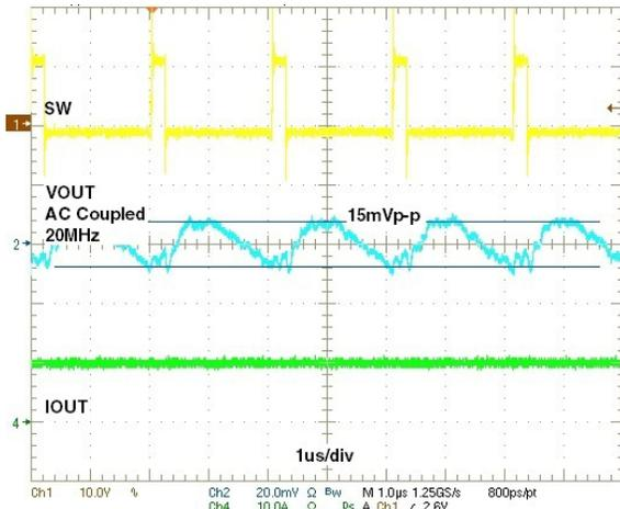
Figure 13: Steady state, CCM,  $I_{OUT} = 10A$
