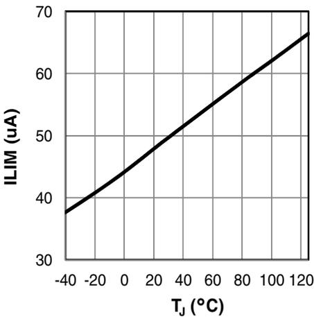
Figure 9:  $I_{LIM}$  versus temperature
