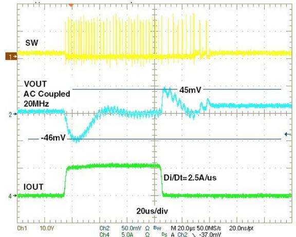
Figure 18: Load step, DCM/CCM, 0A-5A-0A
