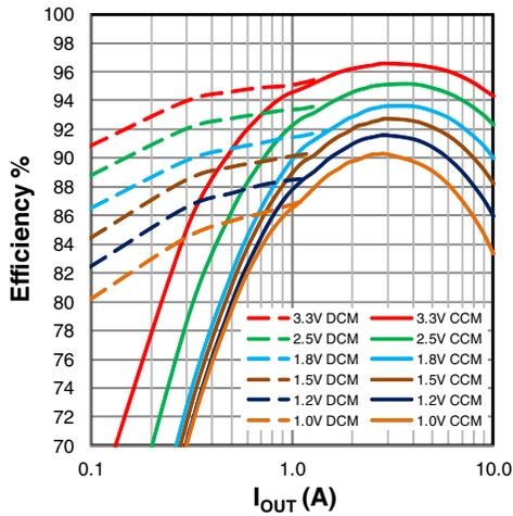
Figure 19: Efficiency,  $V_{IN}=5V$
