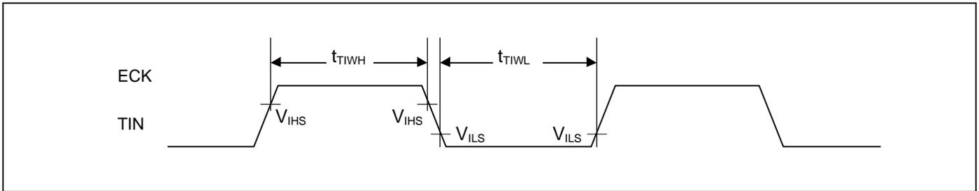
**Trigger input timing**
