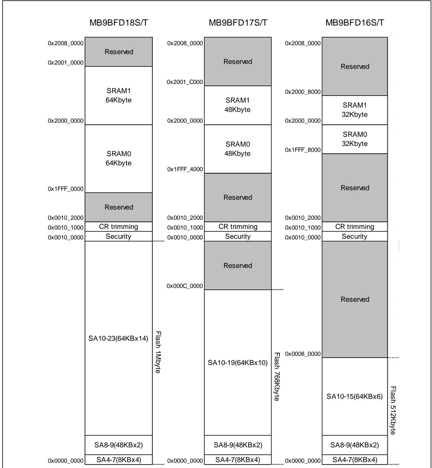
See "MB9BD10T/610T/510T/410T/310T/210T/110T Series Flash programming Manual" for sector structure of Flash.
