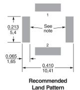
Note: These pads are only for board adhesion. Do not connect these pads to circuit or ground.
