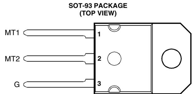
Pin 2 is in electrical contact with the mounting base.
