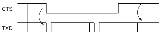
Figure 44-28. Transmitter Behavior when Operating with Hardware Handshaking
