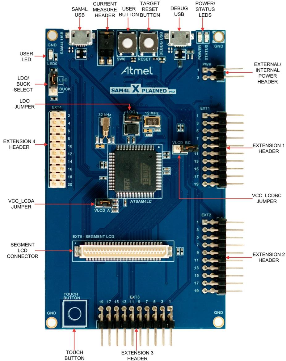
Figure 1-2 SAM4L Xplained Pro Block Diagram
