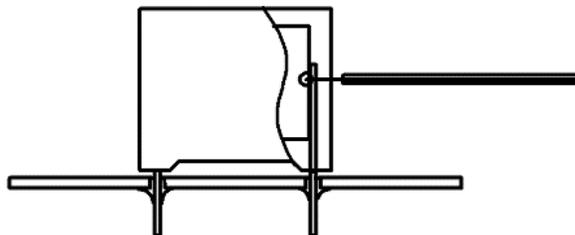
*Temperature monitored inside the capacitor.*
