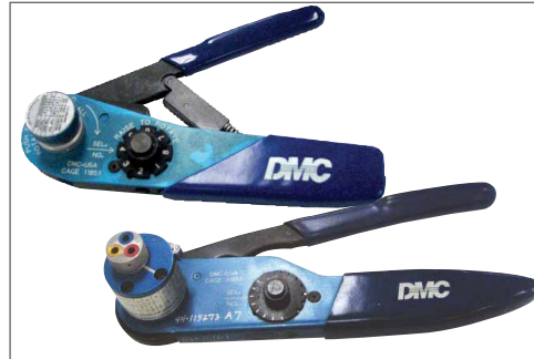
Examples of M22520 Series Crimping Tools: Shown top: tool used for small size 23 contacts. Shown bottom: tool used for size 20, 16 or 12 contacts and has a positioner that can be dialed for each contact size.
