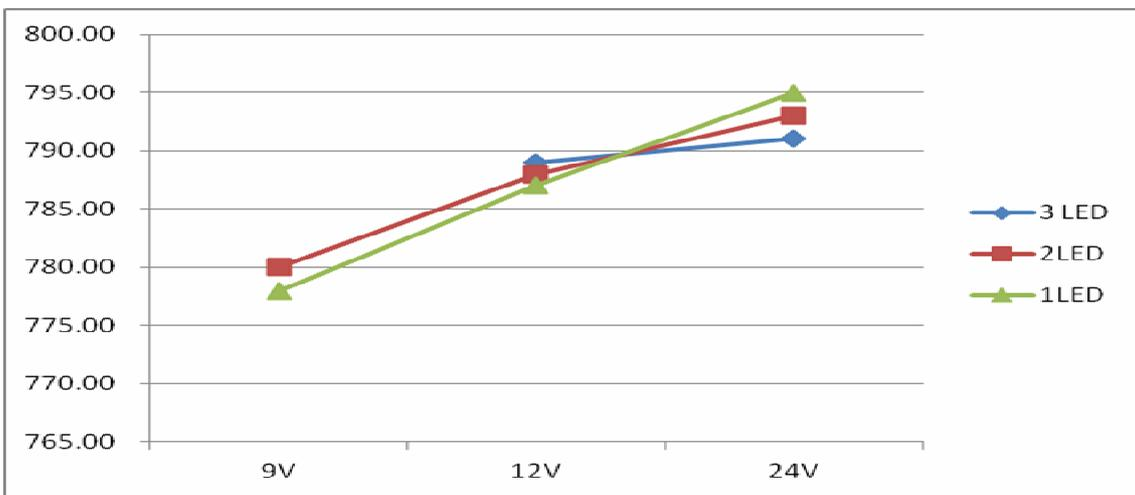
Output current vs. input voltage @L=22uH, I<sub>OUT</sub>=769mA
