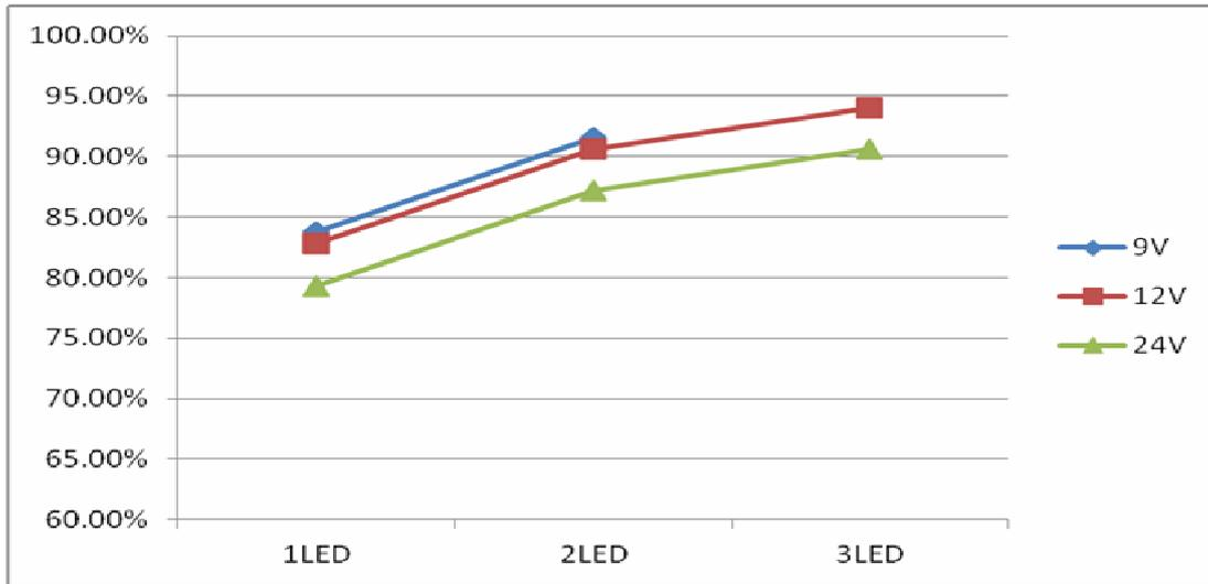
Efficiency vs. LED cascaded number @L=68uH, I<sub>OUT</sub>=769mA
