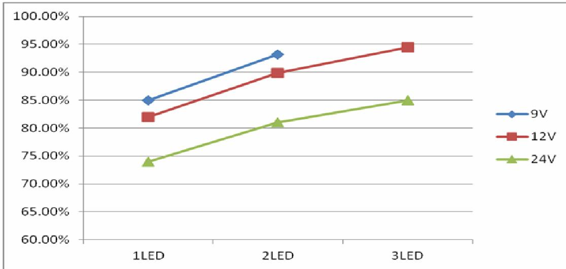
Efficiency vs. LED cascaded number @L=22uH, I<sub>OUT</sub>=384mA
