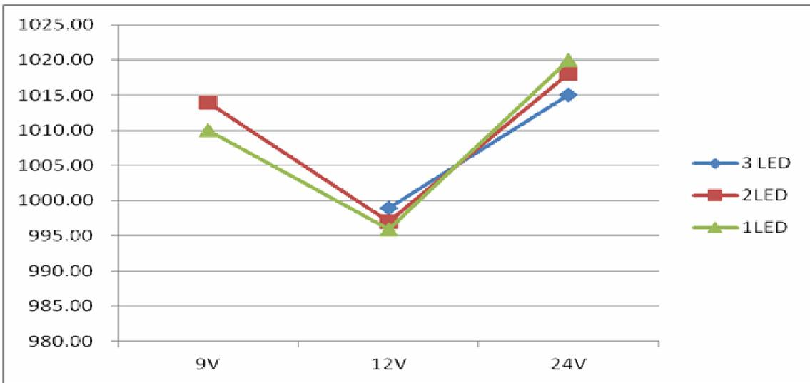
Output current vs. input voltage @L=68uH, I<sub>OUT</sub>=1000mA
