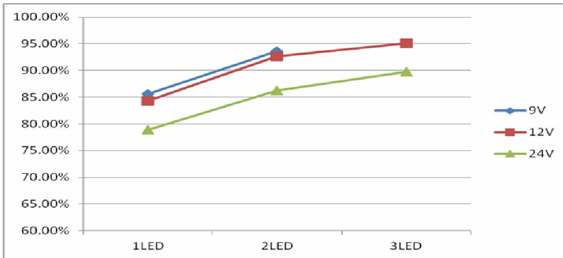
Efficiency vs. LED cascaded number @L=68uH, I<sub>OUT</sub>=384mA
