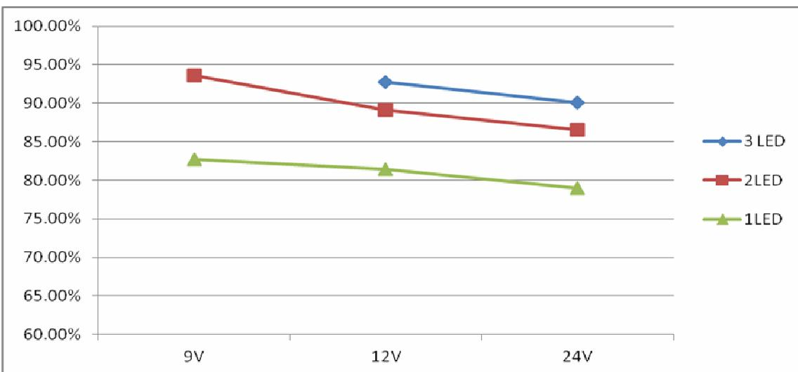
Efficiency vs. input voltage @L=68uH, I<sub>OUT</sub>=1000mA
