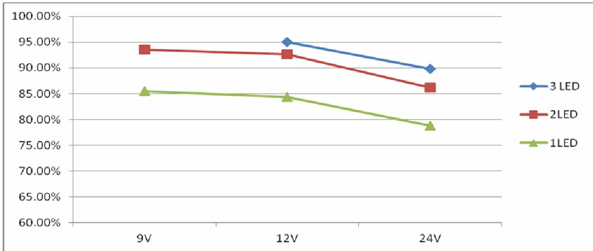
Efficiency vs. input voltage @L=68uH, I<sub>OUT</sub>=384mA
