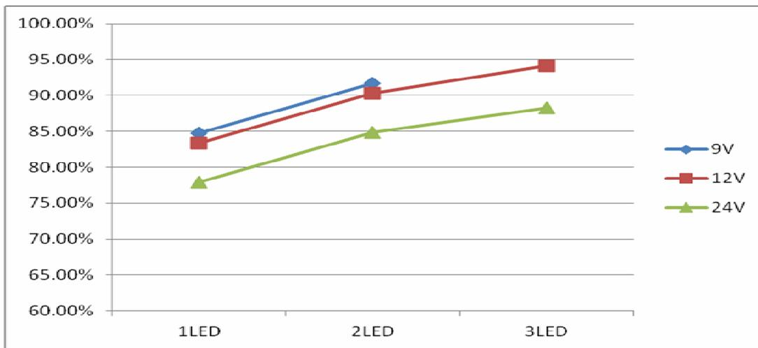
Efficiency vs. LED cascaded number @L=22uH, I<sub>OUT</sub>=1000mA
