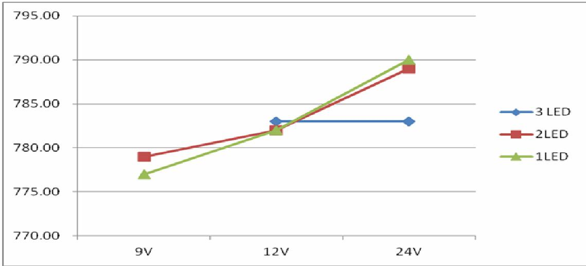
Output current vs. input voltage @L=68uH, I<sub>OUT</sub>=769mA
