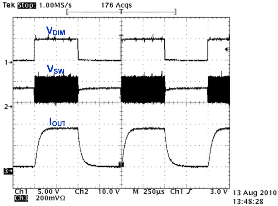
Dimming waveform ( $V_{IN}=12V$ ,  $R_{SEN}=0.27\Omega$ , 3-LED)
