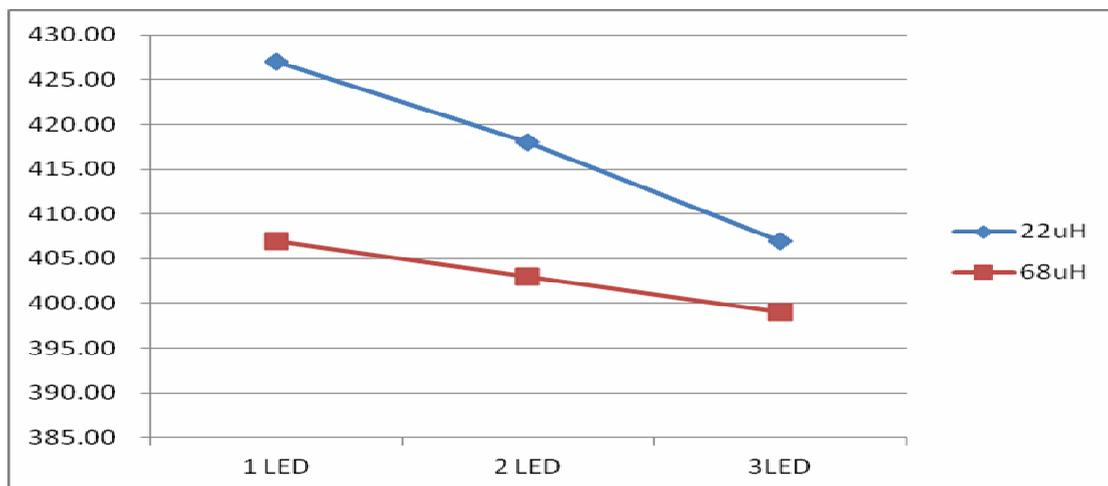
Output Current vs. LED Cascaded number @V<sub>IN</sub>=24V, I<sub>OUT</sub>=384mA
