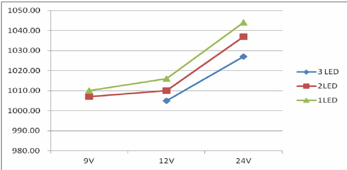
Output current vs. input voltage @L=22uH, I<sub>OUT</sub>=1000mA
