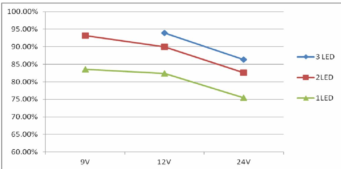
Efficiency vs. input voltage @L=22uH, I<sub>OUT</sub>=769mA
