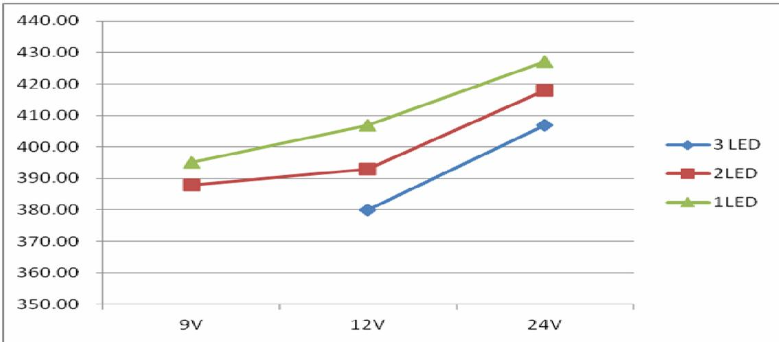
Output current vs. input voltage @L=22uH, I<sub>OUT</sub>=384mA
