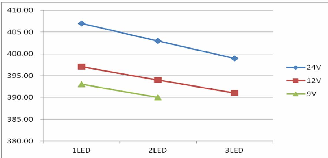
Output current vs. LED cascaded number @L=68uH, I<sub>OUT</sub>=384mA
