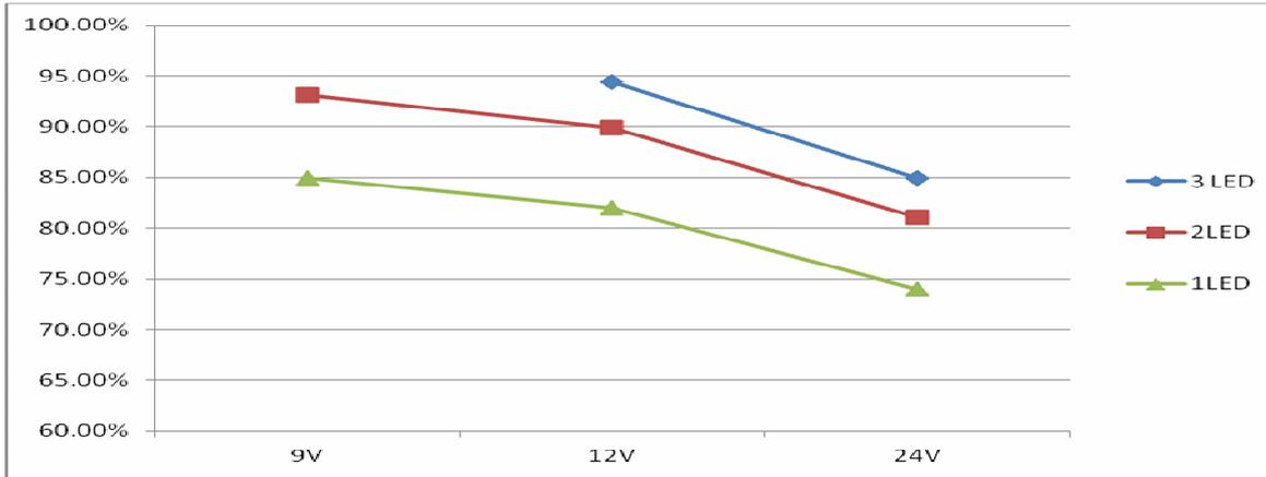
Efficiency vs. input voltage @L=22uH, I<sub>OUT</sub>=384mA
