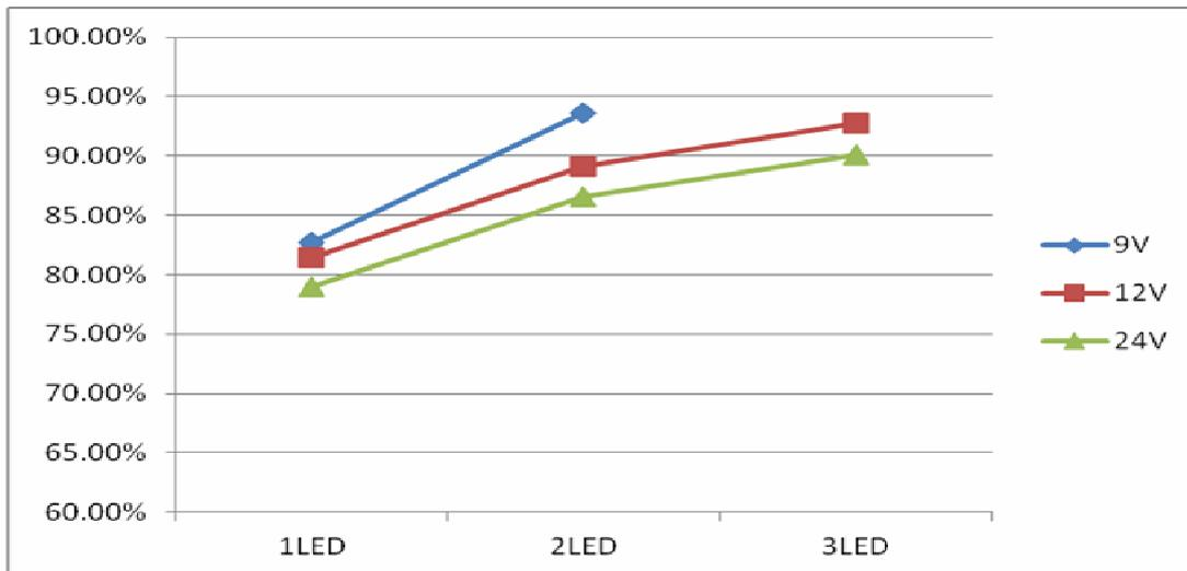
Efficiency vs. LED cascaded number @L=68uH, I<sub>OUT</sub>=1000mA
