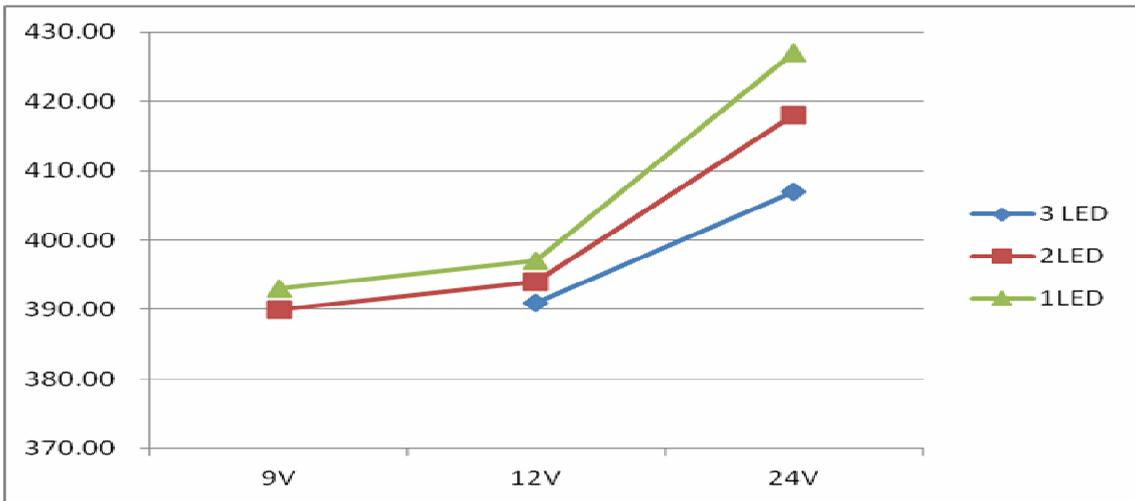
Output current vs. input voltage @L=68uH, I<sub>OUT</sub>=384mA
