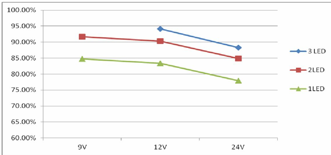
Efficiency vs. input voltage @L=22uH, I<sub>OUT</sub>=1000mA
