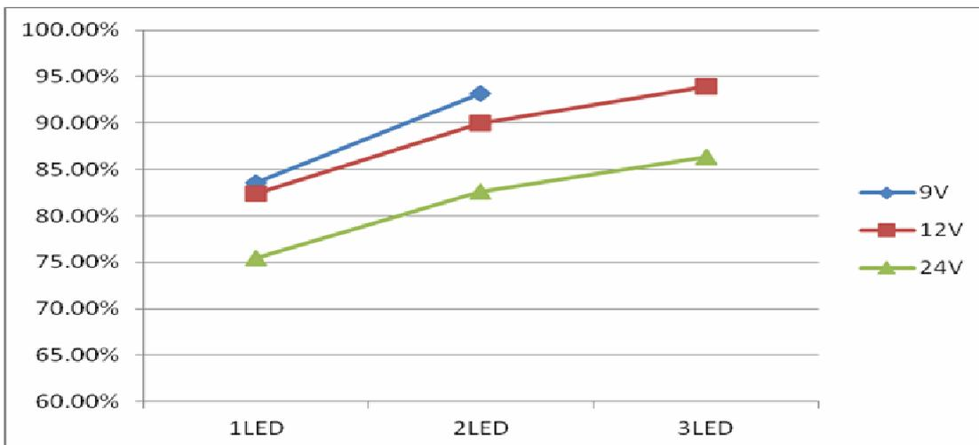
Efficiency vs. LED cascaded number @L=22uH, I<sub>OUT</sub>=769mA
