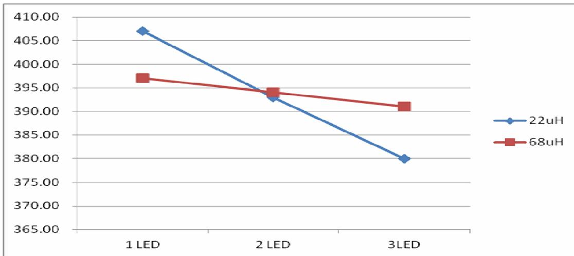
Output Current vs. LED Cascaded number @V<sub>IN</sub>=12V, I<sub>OUT</sub>=384mA
