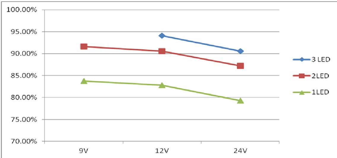
Efficiency vs. input voltage @L=68uH, I<sub>OUT</sub>=769mA
