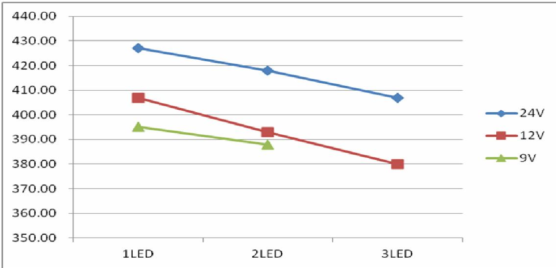
Output current vs. LED cascaded number @L=22uH, I<sub>OUT</sub>=384mA
