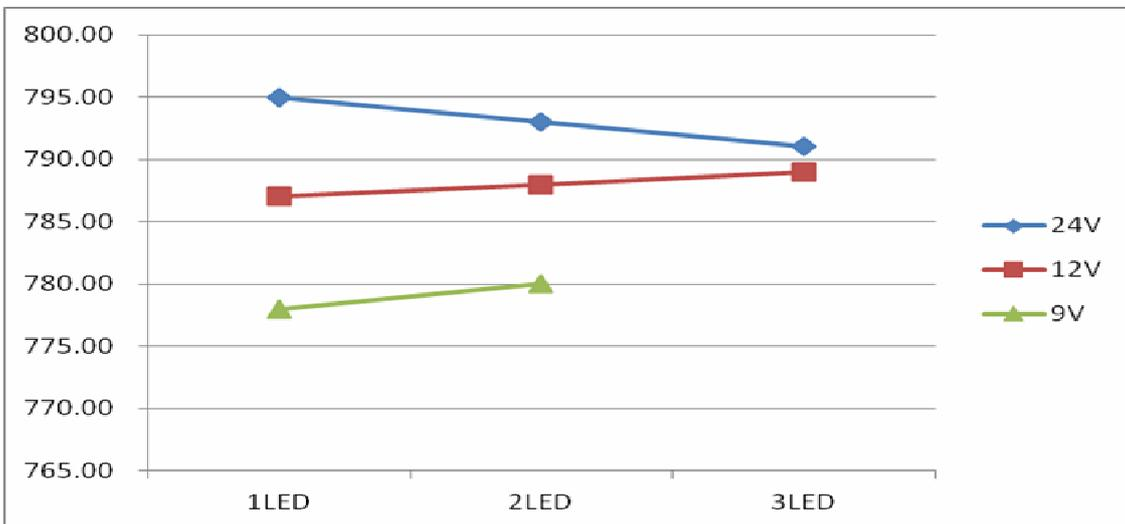
Output current vs. LED cascaded number @L=22uH, I<sub>OUT</sub>=769mA
