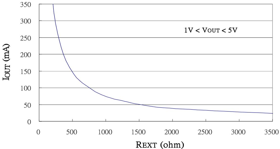
Also, when SCT2004's output voltage is set between 1 Volt and 5 Volt, the output current can be estimated approximately by:  $I_{OUT} = 122(620 / R_{EXT})$  (mA). Thus the output current are all set to be about 84 mA at  $R_{EXT} = 900 \Omega$ .
