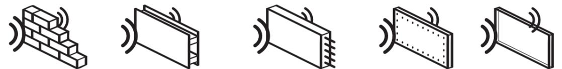
bricks: from 10 to 40 %, wood and plaster: from 5 to 20 %, reinforced concrete: from 40 to 80 %, metal: from 90 to 100%, glass: from 10 to 20 %
