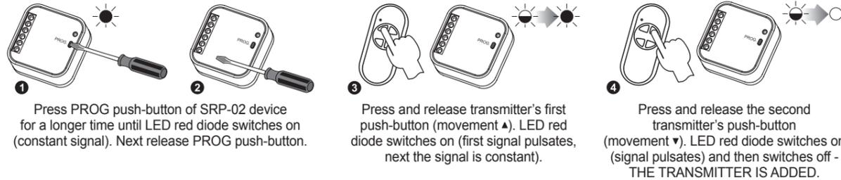
1 Press PROG push-button of SRP-02 device for a longer time until LED red diode switches on (constant signal). Next release PROG push-button.
