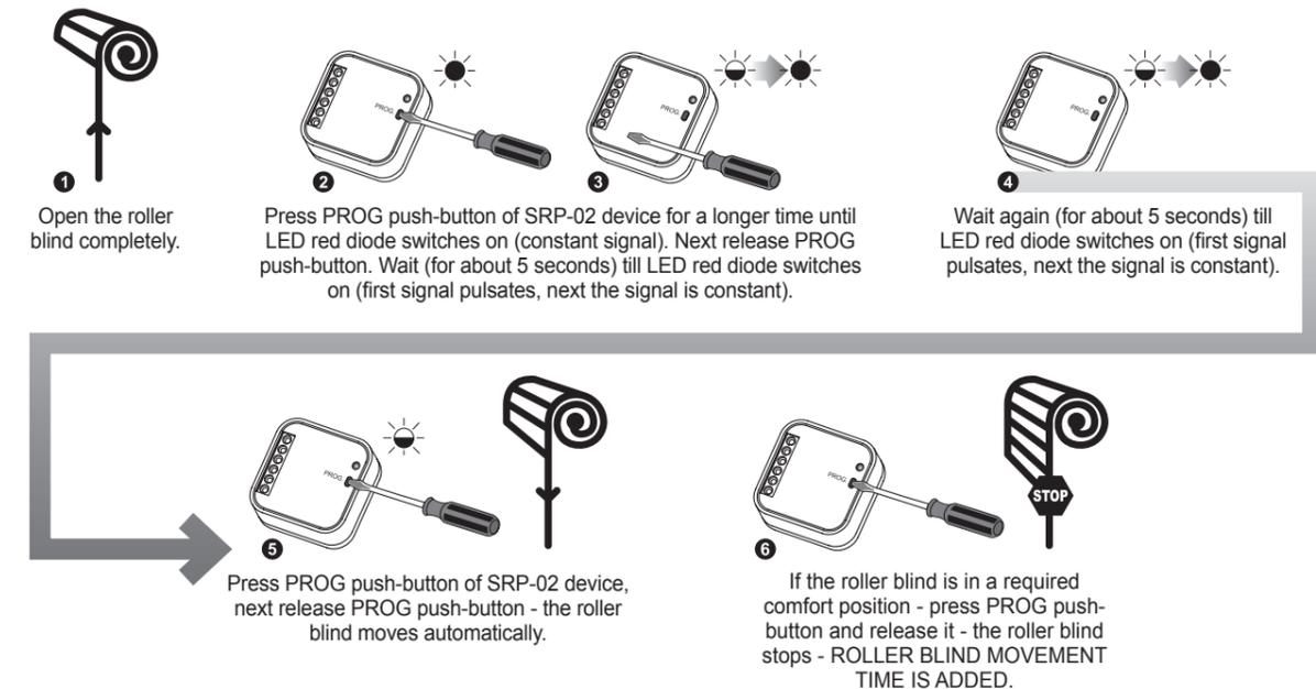
Time programming example for upper comfort mode. In order to programme time for bottom comfort mode, it is necessary to close the roller blind completely before programming procedure starts. Maximum time is 120 seconds.
