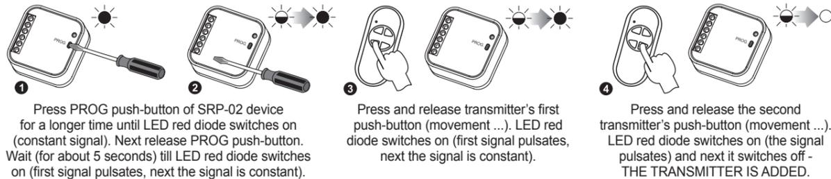
1 Press PROG push-button of SRP-02 device for a longer time until LED red diode switches on (constant signal). Next release PROG push-button. Wait (for about 5 seconds) till LED red diode switches on (first signal pulsates, next the signal is constant).
