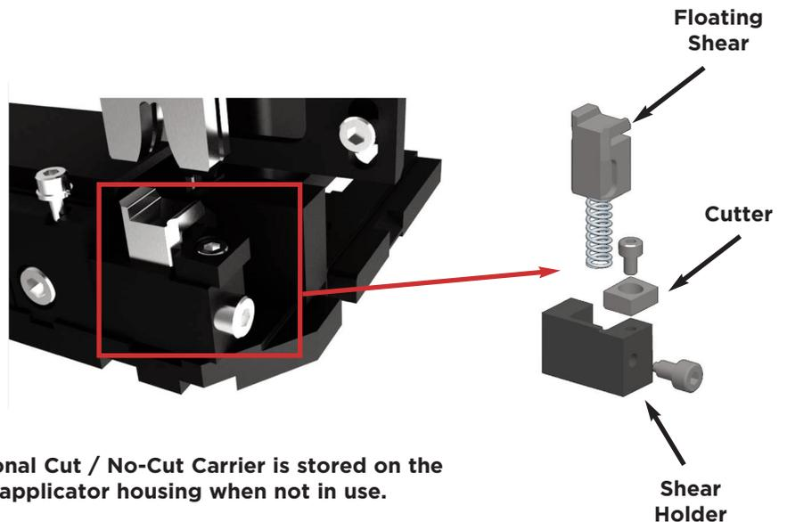
Optional Cut / No-Cut Carrier is stored on the applicator housing when not in use.
