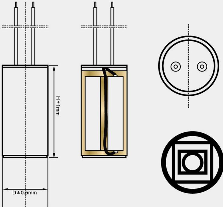
Motor run capacitor Dimensions:
