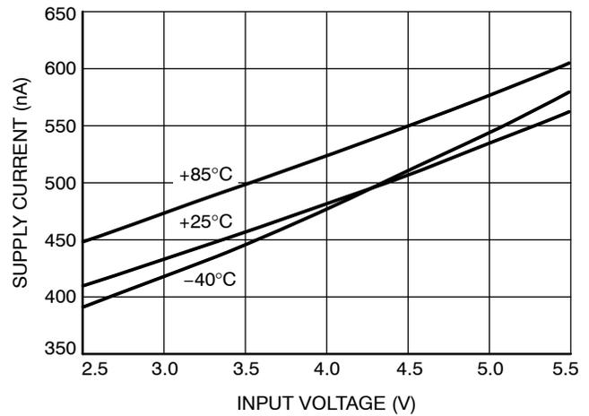
Figure 3. Supply Current vs. Input Voltage Over Temperature
