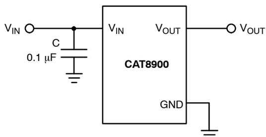
Figure 1. Application Circuit
