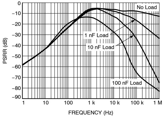
Figure 13. Power Supply Rejection Ratio vs. Frequency
