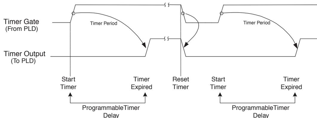
Note that if the clock module is configured as “slave” (i.e. the CLK is an input), the actual time-out of the two timers is determined by the external clock frequency.
