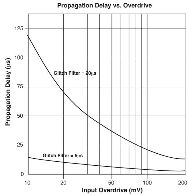
Note: Typical propagation delay of V<sub>MON</sub> inputs to outputs as a function of overdrive beyond selected trip point.
