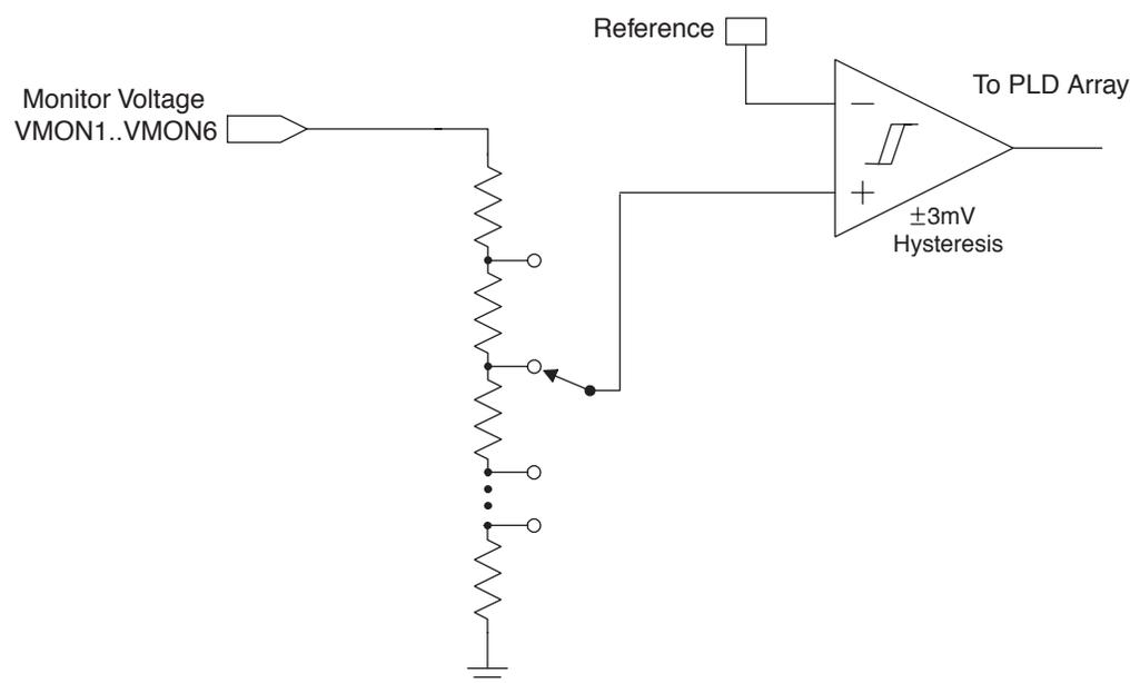
Each monitor consists of three major subsystems. The core of the monitor is a voltage comparator. This comparator outputs a HIGH signal to the PLD array if the voltage at its positive terminal is greater than that at its negative terminal, otherwise it outputs a LOW signal. A small amount of hysteresis is provided by the comparator to reduce the effects of input noise.
