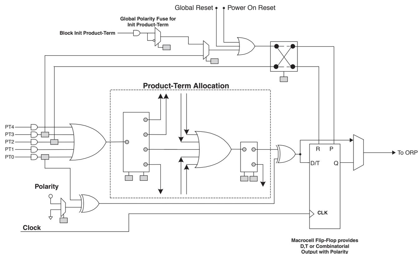
Figure 4. PLD and Timer Functional Block Diagram
