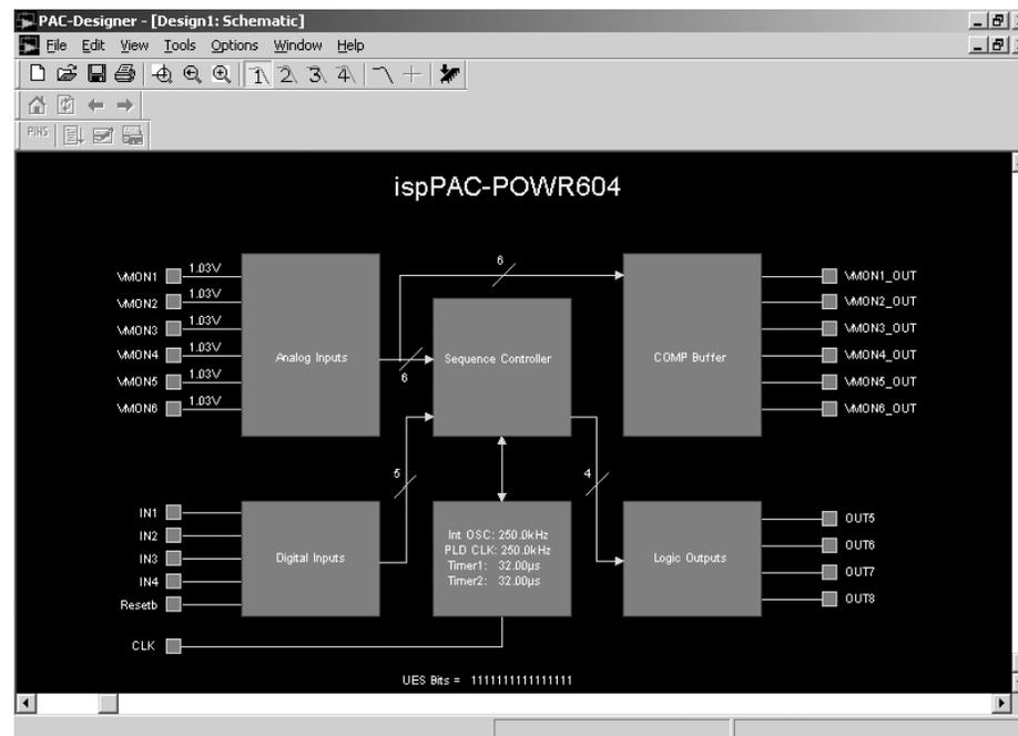
The user interface (Figure 14) provides access to various internal function blocks within the ispPAC-POWR604 device.
