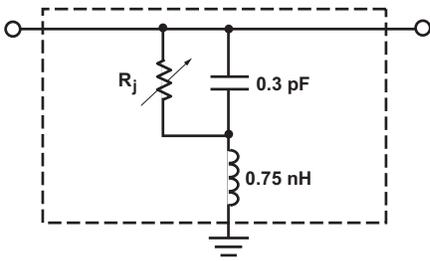
Figure 11. Equivalent Circuit.
