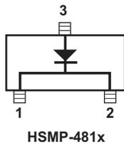
Figure 6. Internal Connections.
