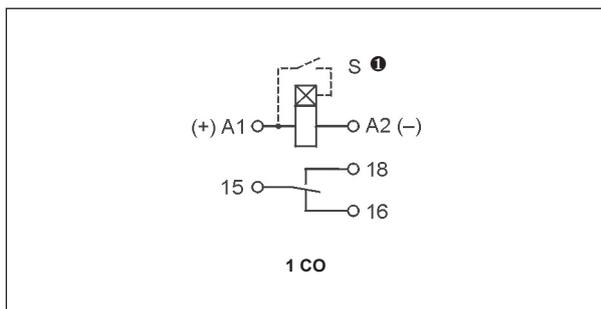
❶ The control terminal S is activated by connection to A1 terminal via the external control contact S.
