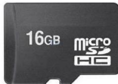
Support is available for off-the-shelf high capacity HC memory cards (4GB and above). Memory cards up to 32GB in size can be used, as FAT16 or FAT32, however it must be noted that only a portion of this can be utilised by the FAT16 file system.
