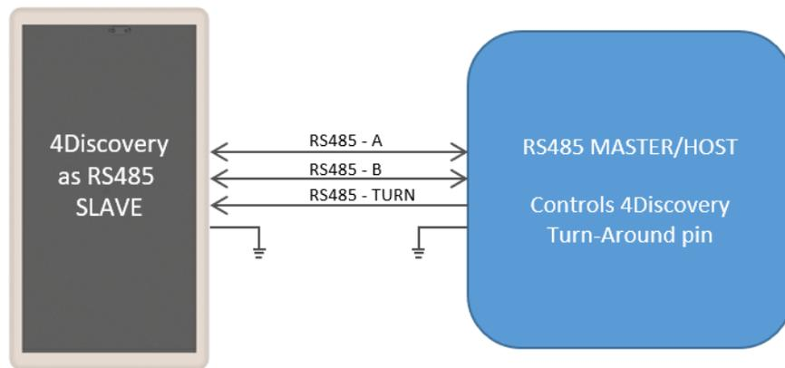
This image shows the 4Discovery when acting as a Slave, where the Master device is controlling the Turn pin of the 4Discovery. This is an unlikely situation, as the 4Discovery typically would be programmed to Auto Turn based on the protocol of the Master.
