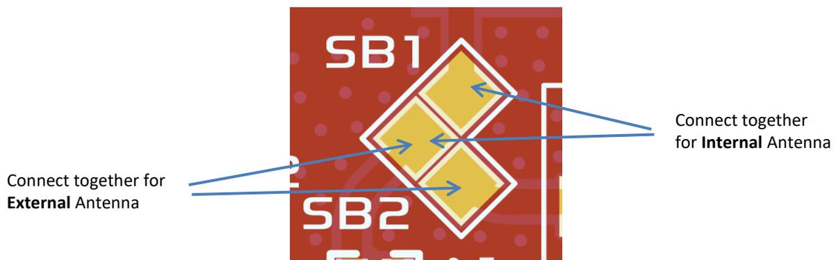
**Note:** If both SB1 and SB2 are connected at the same time, then WiFi performance may be impacted, as both the internal and the external antenna will be enabled at the same time.
