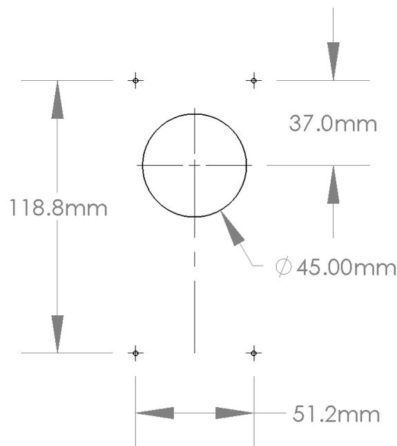
The 4 corner holes are actually slots on the plastic, which give some tolerance when mounting. The slots actually allow for 51.15mm to 56.15mm horizontal centres.
