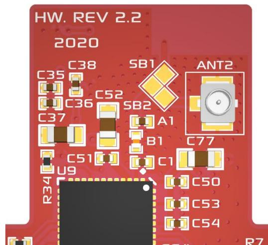
By default, SB1 is soldered closed with a solder blob, which enables the ESP32 to be connected to the internal antenna on the rear side of the PCB.
