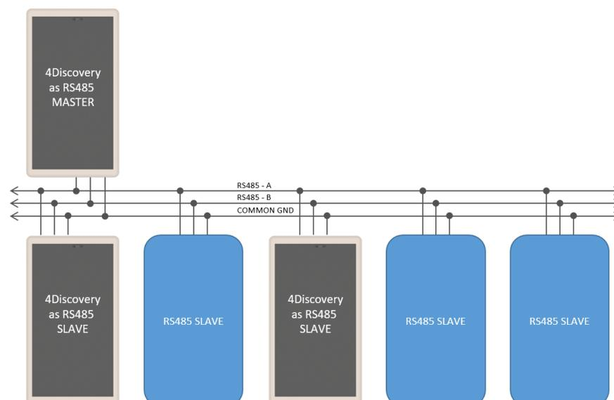
Figure 1. Typical 2-wire RS485 configuration, which includes a common ground.
