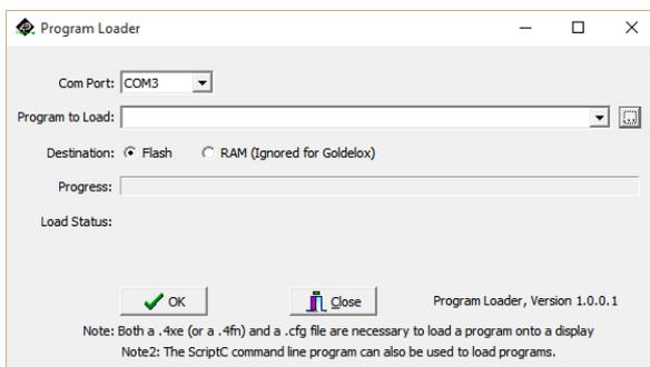
**ScriptC** is a command line interface which can be controlled from a Batch Script or similar, useful for repetitive loading or when controlled from an external application. Example scripts are provided, showing how to load PmmC, Display Drivers and Applications using a batch script.
