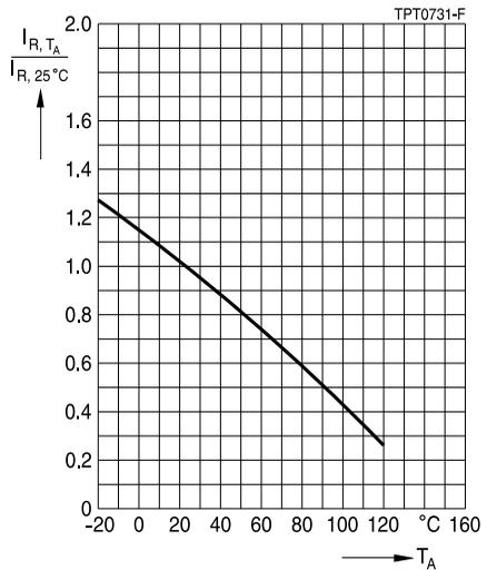
**Characteristics (typical) for  $T_{ref} = 120\text{ }^{\circ}\text{C}$**
