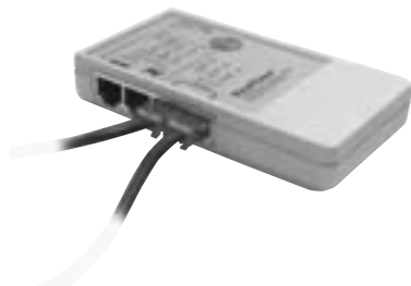
AX-110BT Realtime 10/100 Base-TX Ethernet Network Test Unit
