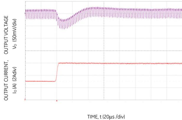
Figure 22. Transient Response to Dynamic Load Change on one output from 50% to 100% at 12Vin, C<sub>out</sub> = 2x47µF + 1x330µF, C<sub>Tune</sub> = 1500pF & RT<sub>une</sub> = 300Ω
