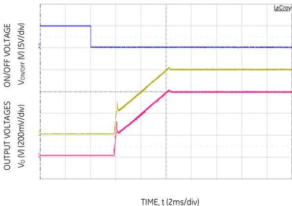
Figure 5. Typical Start-up Using On/Off Voltage (V<sub>IN</sub>=12V, I<sub>o</sub> = I<sub>o1,max</sub>, I<sub>o2,max</sub>).
