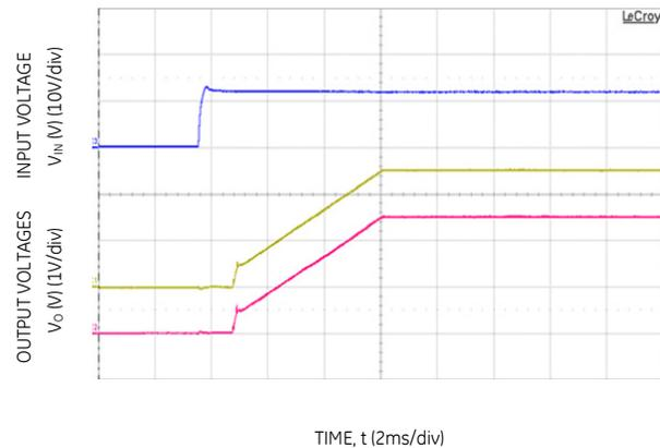
Figure 24. Typical Start-up Using Input Voltage (V<sub>IN</sub> = 12V, I<sub>o</sub> = I<sub>o1,max</sub>, I<sub>o2,max</sub>).
