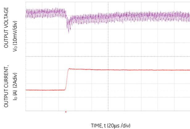
Figure 4. Transient Response to Dynamic Load Change from 50% to 100% on one output at 12Vin, C<sub>out</sub>=3x47µF+3x330µF, C<sub>Tune</sub>=12nF, R<sub>Tune</sub>=300Ω
