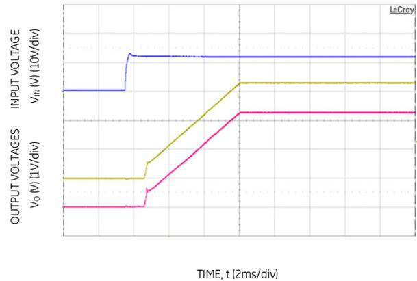
Figure 30. Typical Start-up Using Input Voltage (V<sub>IN</sub> = 12V, I<sub>o</sub> = I<sub>o1,max</sub>, I<sub>o2,max</sub>).
