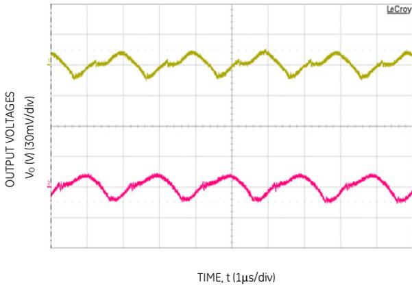
Figure 27. Typical output ripple and noise (C<sub>o</sub>= 2x4.7nF+2x47µF ceramic, V<sub>IN</sub> = 12V, I<sub>o</sub> = I<sub>o1,max</sub>, I<sub>o2,max</sub>).
