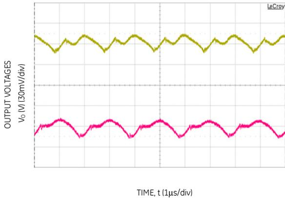
Figure 21. Typical output ripple and noise (C<sub>0</sub>= 2x4.7nF+2x47µF ceramic, V<sub>IN</sub> = 12V, I<sub>o</sub> = I<sub>o1,max</sub>, I<sub>o2,max</sub>).
