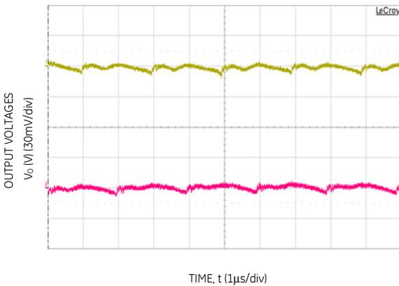
Figure 3. Typical output ripple and noise (C<sub>O</sub>= 2x4.7nF+2x47µF ceramic, V<sub>IN</sub> = 12V, I<sub>o</sub> = I<sub>o1,max</sub>, I<sub>o2,max</sub>).
