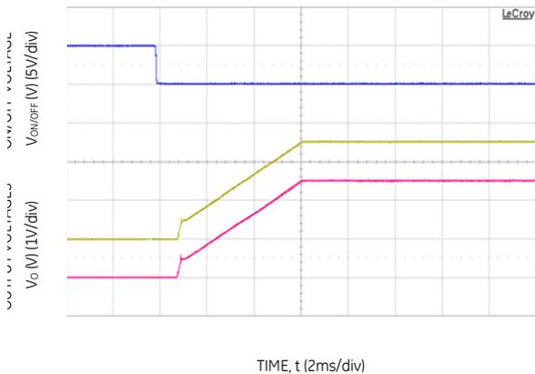
Figure 23. Typical Start-up Using On/Off Voltage (V<sub>IN</sub> = 12V, I<sub>o</sub> = I<sub>o1,max</sub>, I<sub>o2,max</sub>).
