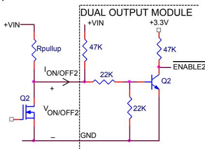
Figure 39. Circuit configuration for using positive On/Off logic.
