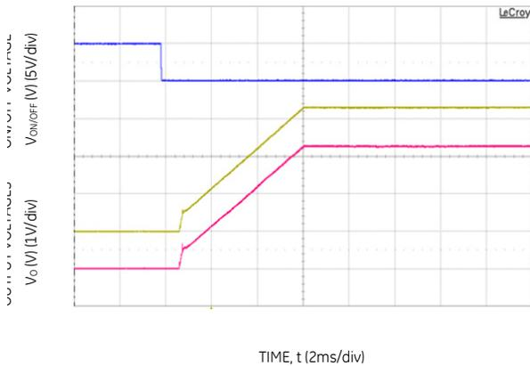
Figure 29. Typical Start-up Using On/Off Voltage (V<sub>IN</sub> = 12V, I<sub>o</sub> = I<sub>o1,max</sub>, I<sub>o2,max</sub>).
