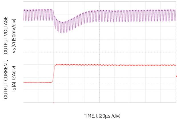
Figure 28 Transient Response to Dynamic Load Change on one output from 50% to 100% at 12V<sub>in</sub>, C<sub>out</sub> = 2x47µF+1x330µF, C<sub>Tune</sub> = 1200pF & R<sub>Tune</sub> = 300Ω
