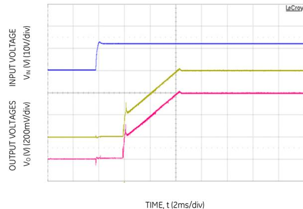
Figure 6. Typical Start-up Using Input Voltage (V<sub>IN</sub> = 12V, I<sub>o</sub> = I<sub>o1,max</sub>, I<sub>o2,max</sub>).
