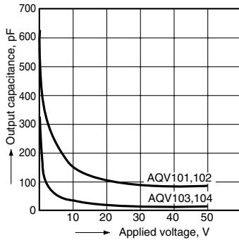
11.-2 Output capacitance vs. applied voltage characteristics (AC/DC type)
