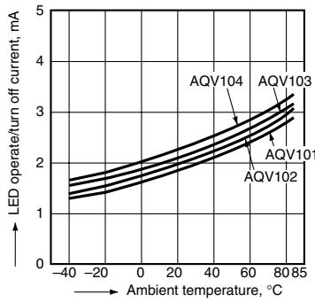
5.-2) LED operate/turn off current vs. ambient temperature characteristics (AC/DC type)
