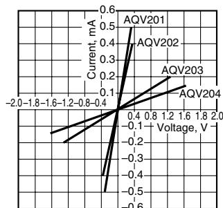
8. Off state leakage current vs. load voltage characteristics
