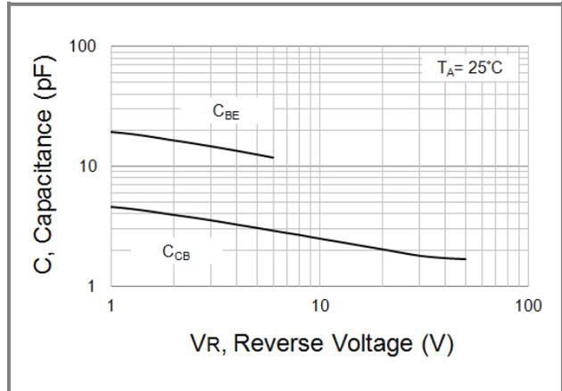
Fig.4 Typical Capacitance
