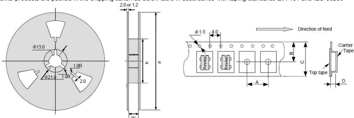
Standard Packing Quantity & Dimension(Unit mm)
