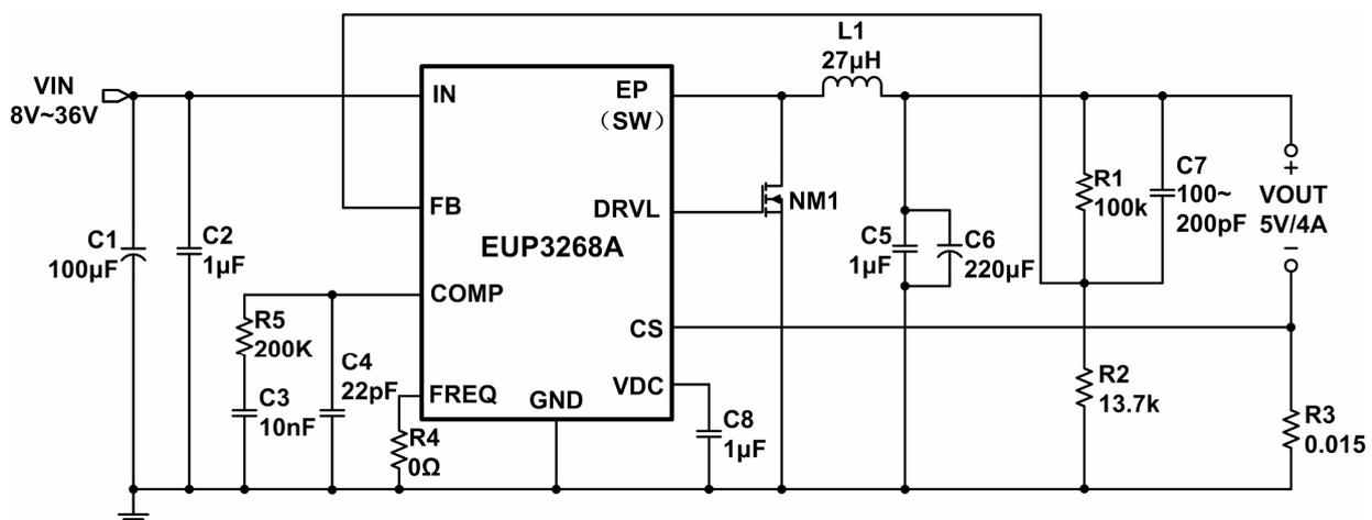
Figure 1. Application Circuit
