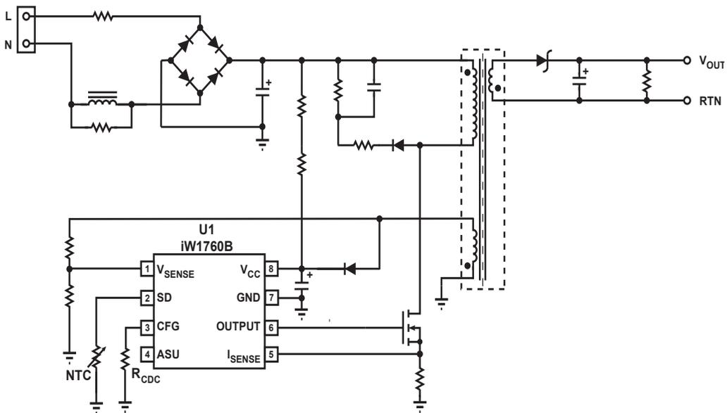
**Figure 3.2 : iW1760B Typical Application Circuit
