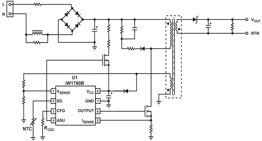
**Figure 3.1 : iW1760B Typical Application Circuit
