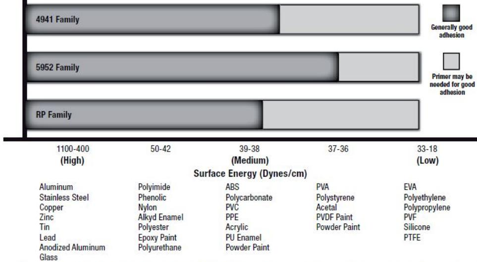
**NOTES:** There are a wide variety of formulations, surfaces finishes and surface treatments available on substrate materials which can affect adhesion. This chart is intended to provide only a rough estimate of the adhesion levels which can be expected on some common materials relative to a reference surface such as aluminum. Foam type can affect and/or limit maximum adhesive strength.
