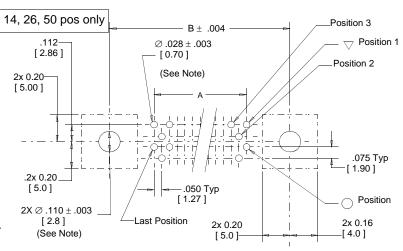
Note: Plated through holes for .062  $\!\!^{\prime\prime}$  board thickness.
